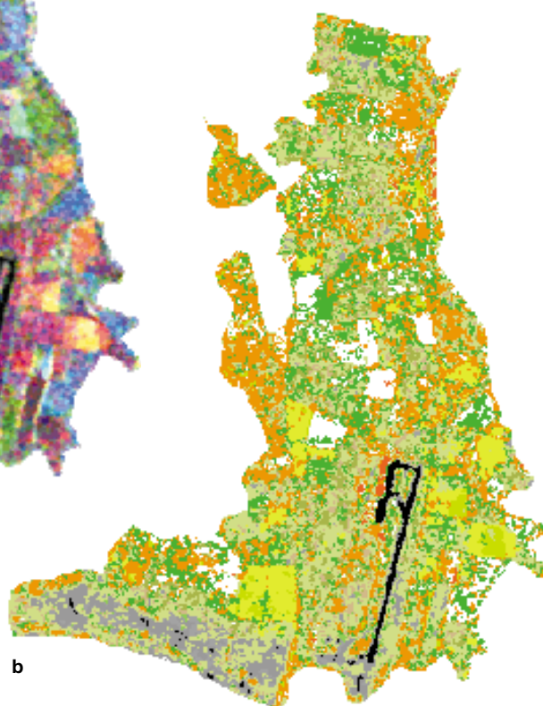
Figure 2f. (a) Multi-temporal SAR image of the land-use-mapping test area (red: data acquired in August, green: in March, blue: in May); (b) Classification results
