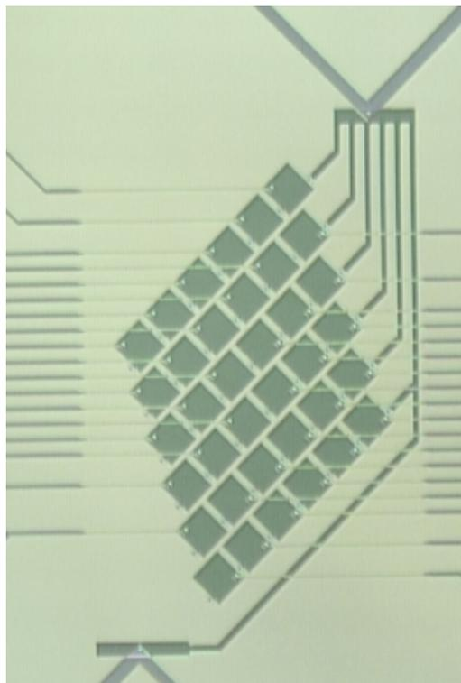
**Figure 1. Optical microscope photograph of the 6 x 6 array**
