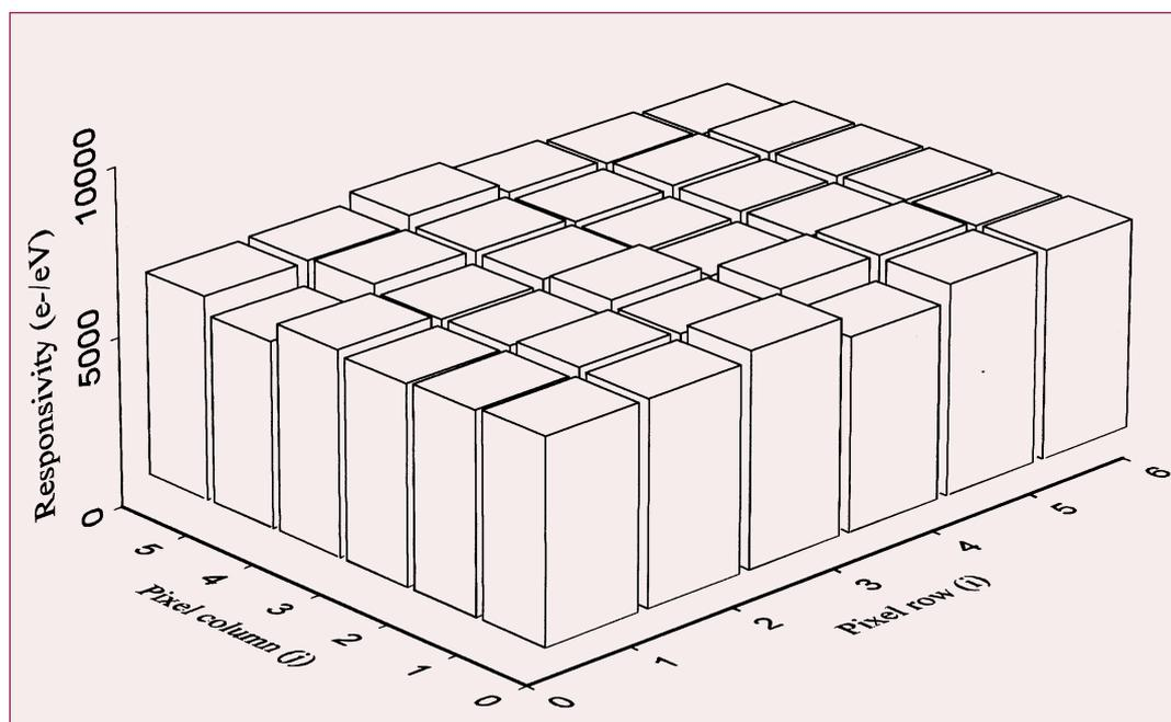
**Figure 2. Mapping of the array's responsivity (36 elements)**
