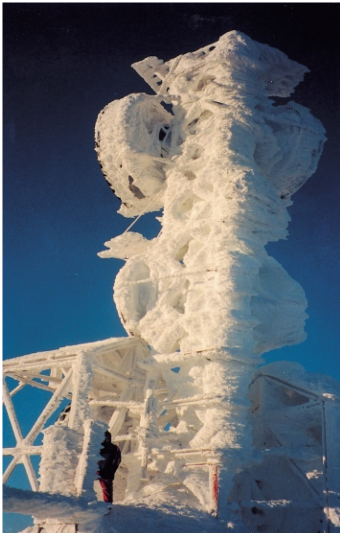
Figure 9. The Monkey Hill test site showing the rime-ice-encrusted test panel (left)
