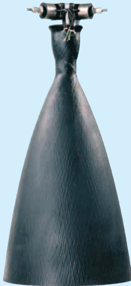
Model of the novel European 500 N spacecraft apogee motor developed for AlphaBus by EADS-ST (D)
