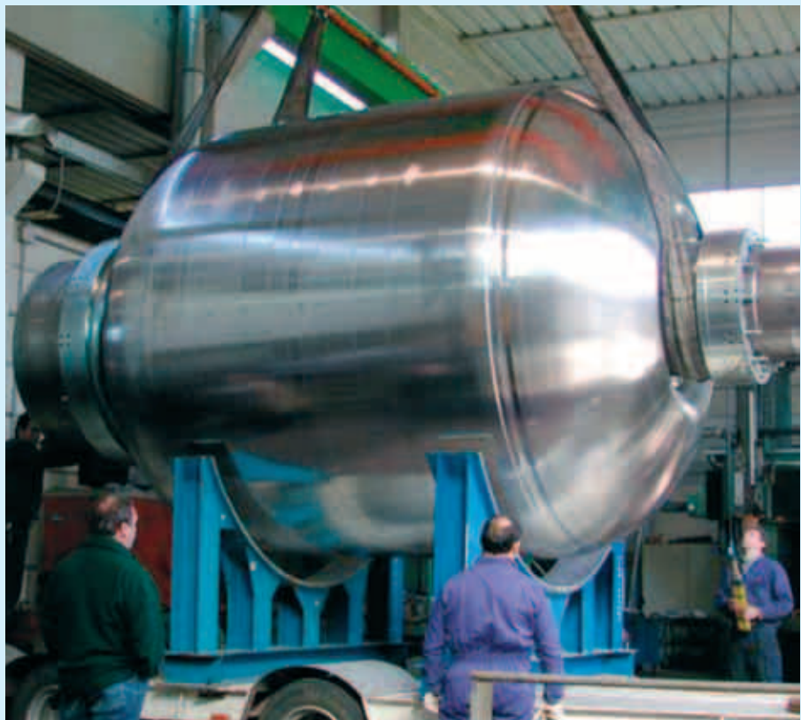
The winding mandrel for the technological model of the P80 motor, which constitutes Vega's first stage (Photo courtesy of Avio)
