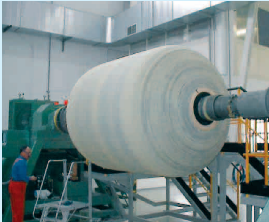
Manufacture of the Zefiro-9 development model in progress at Colleferro (I). This solid-propellant motor is the main component of Vega's third stage (Photo courtesy of Avio)
