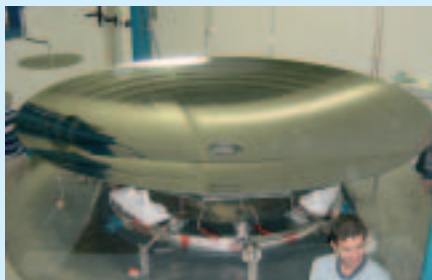
The Herschel telescope's primary mirror polished at Opteon in Finland
