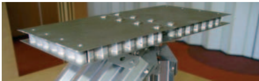
Reusable rudder metallic structure building-block element (Courtesy of Dutch Space)
