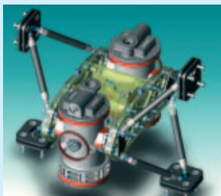
The LISA Technology Package Central Assembly, showing the two inertial sensors, containing the proof masses, the Zerodur optical bench and side slabs supported by eight carbon fibre struts
