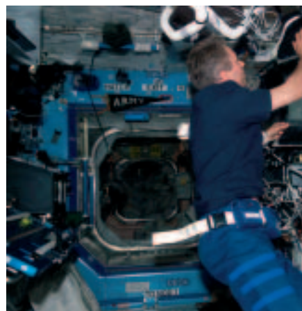
Astrolab: Thomas Reiter working on the Pulmonary Function System in Destiny. ESA provided the PFS for the Human Research Facility
