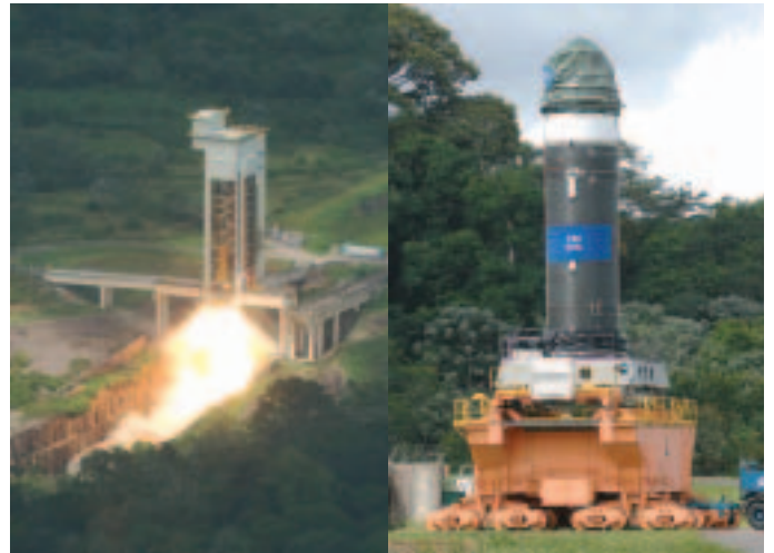
Vega's P80 first-stage motor roared to life for the first time on 30 November 2006 when demonstration motor DM-1 was tested (left) in Kourou, French Guiana. This successful firing will be followed by a second and final test in mid-2007. Right: DM-1 is transferred to the test stand. (ESA/CNES-SOV)
