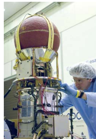
Right: the 5.5 kg, 40 cm-diameter YES2 capsule will be the first space payload to use a tether to begin its return to Earth
