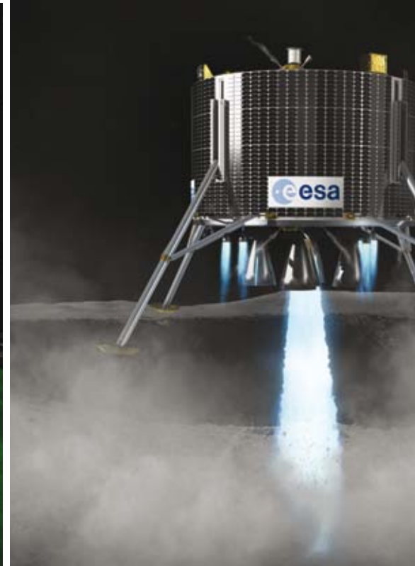
↑ Thrust is reduced for final phases of terminal descent (ESA/AOES Medialab)
