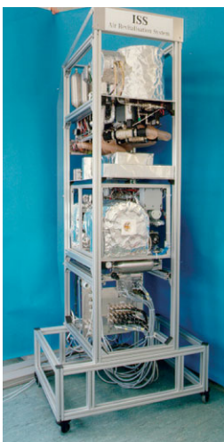
The ARES Demonstrator Unit. CO 2 Concentration (top), CO 2 Reduction (middle) and Oxygen Generation in a half-width ISS Rack.
