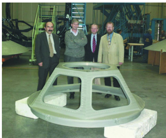
Fig. 1. Produced from a single forging, Cupola's dome requires no welds. The fully machined forging for the Qualification Model is shown. From left: L. Basile (Alenia), D. Laurini, C. Soulez-Lariviere and G. Woop (ESA).
