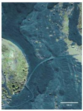
Fig. 13. This test image, looking across Lake Constance in March 1995, illustrates HRSC's resolution. The cable car rope (diameter 10-15 cm) is imaged from a distance of 40 km. The pixel resolution at this range is 1.6 m.
