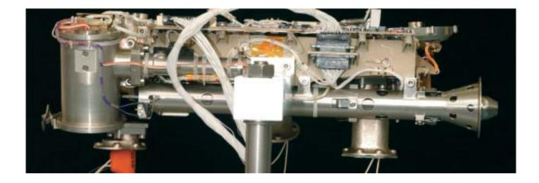
Fig. 10. The PLUTO FM mounted on the PAW FM. The Mole is just visible at the right, protruding from the launch tube (minus the sampling head, which is fitted as late as possible to avoid biological contamination). The winch housing is the cylindrical object on the left. *All Rights Reserved, Beagle 2*  Table 7. PLUTO engineering parameters.
