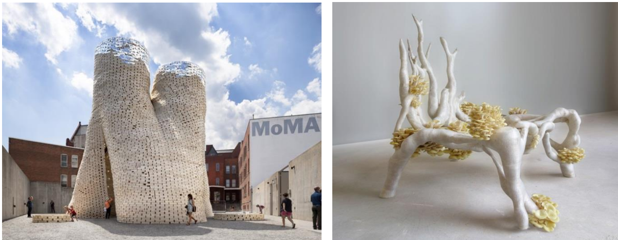
Figure 1. Mycelium bricks used as a structural material in 'Hy-Fi' by The Living (left) [13] [14] and 3D printed 'Mycelium Chair' by Eric Klarenbeek (right) [15]
