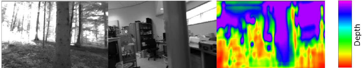
Figure 1. Even with large, varying training data sets, learned capabilities may generalize poorly to a robot’s actual real-world environment. Left: Image used in ref[2]. Middle: image from our lab at TU Delft. Right: application of the trained deep network from ref[2] on the lab image. Colormap indicates that purple / blue represents large distances, while red/yellow is close by. The distance to the large pillar (the closest obstacle) is estimated very badly and would likely lead to a collision in a navigation task. Figure 1. Even with large, varying training data sets, learned capabilities may generalize poorly to a robot’s actual real-world environment.
