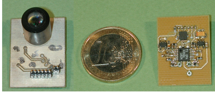
Figure 3: An example of OF sensor based on the Franceschini's scheme. Adapted from [19]
