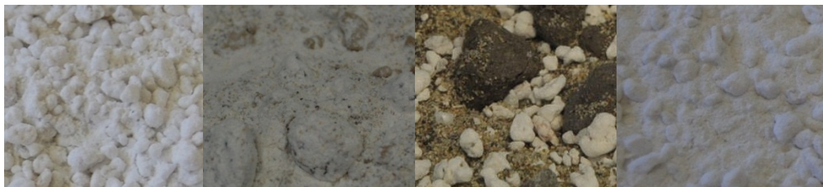
Fig. 7 Overview of all the soils used to test the self-burial performance of Erodium Cicutarium seeds. From the left to the right: Moon, Mars, Asteroid and Test soil.
