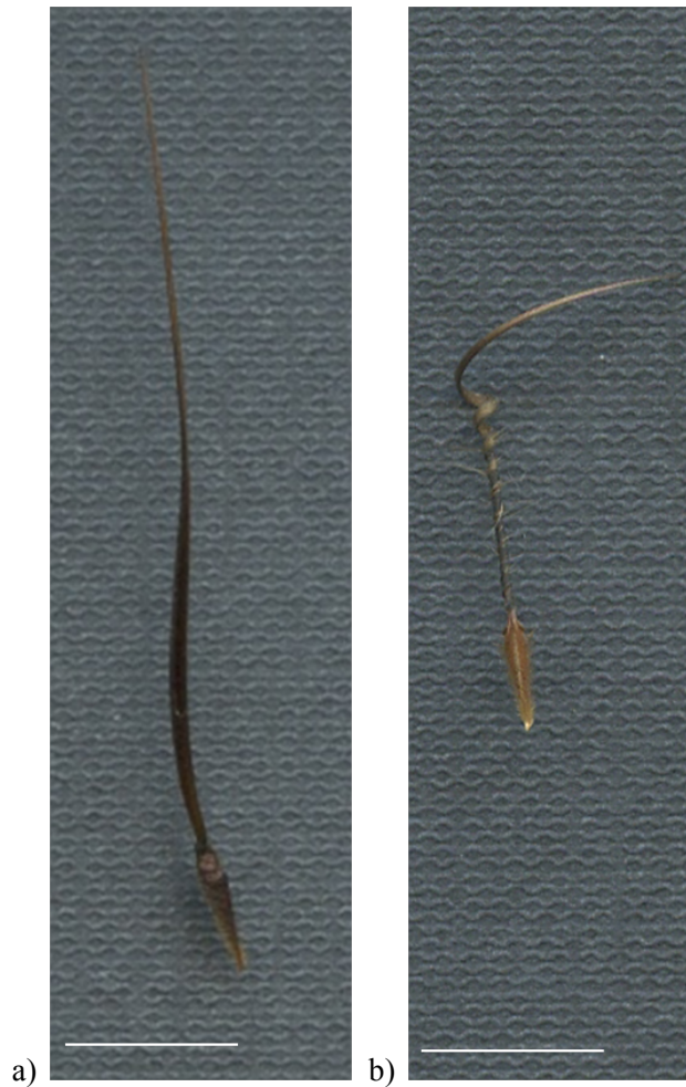
Fig. 56 a) Whet awn corresponding to the initial configuration and b) dry awn corresponding to the final configurations (scale bar – 1 cm).
