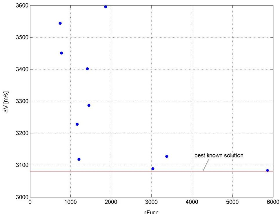
Figure 251: Distribution of the final solutions corresponding to each optimization run on the  $nFunc-\Delta V$  plane.
