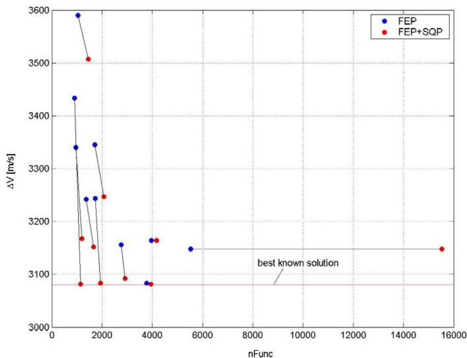
**Figure 279:** Distribution of the improved solutions at the end of a local optimization process on the  $nFunc$ - $\Delta V$  plane.
