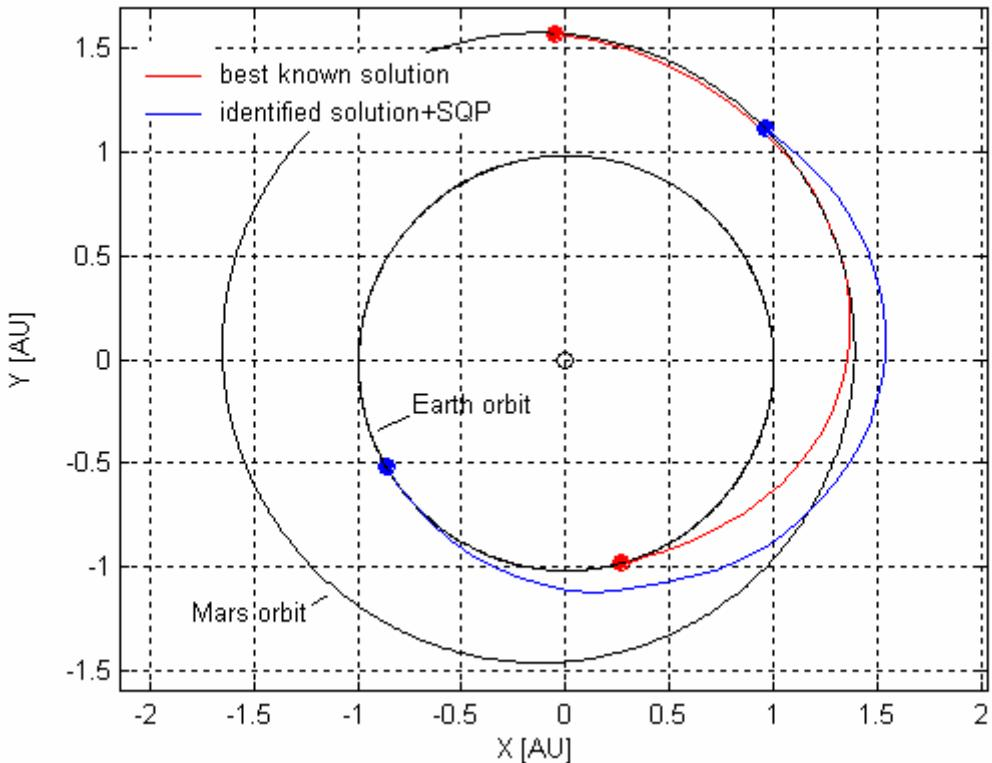
**Figure 236:** Comparison between solution resulting from glbSolve+SQP run and the best known solution in terms of transfer trajectory.
