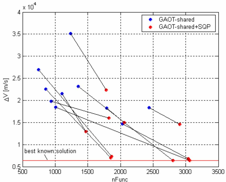
**Figure 168:** Comparison between solutions resulting from GAOT-shared runs and their improvements by means of a further local optimization process via SQP algorithm over the  $nFunc - \Delta V$  plane.
