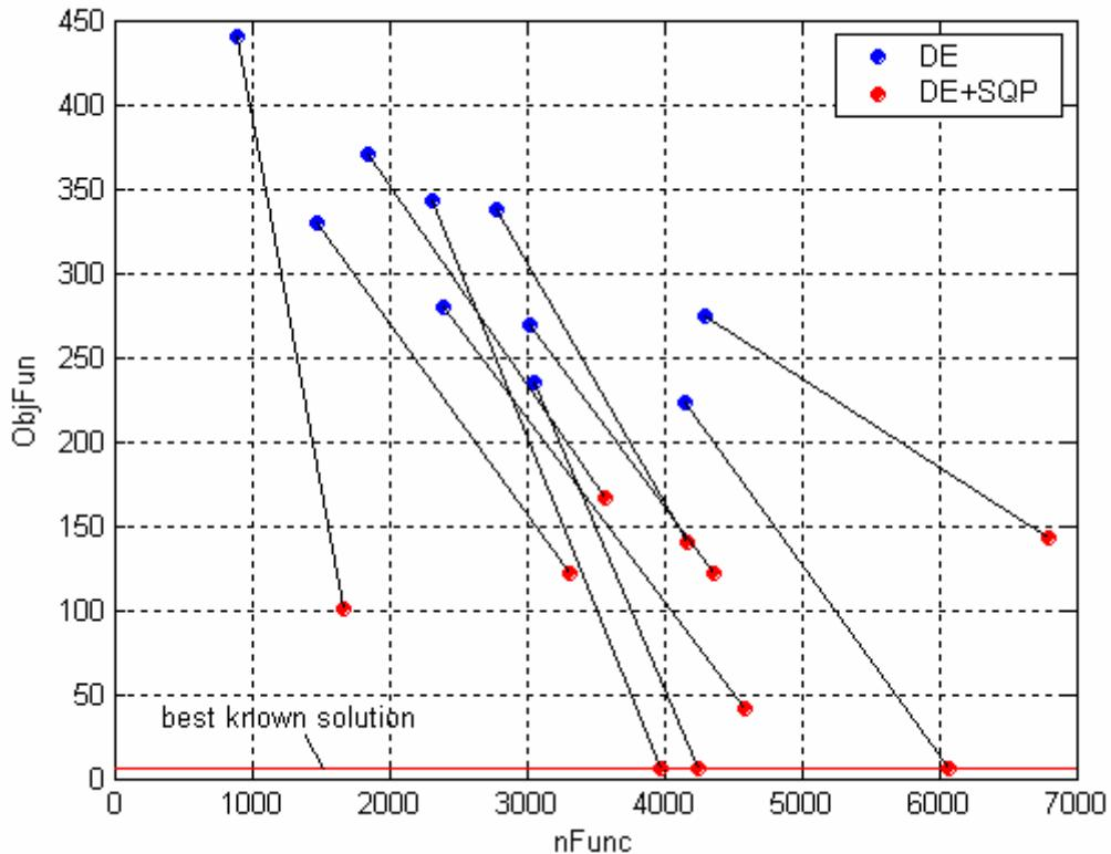
**Figure 226:** Comparison between solutions resulting from DE runs and their improvements by means of a further local optimization process via SQP algorithm over the  $nFunc - \Delta V$  plane.
