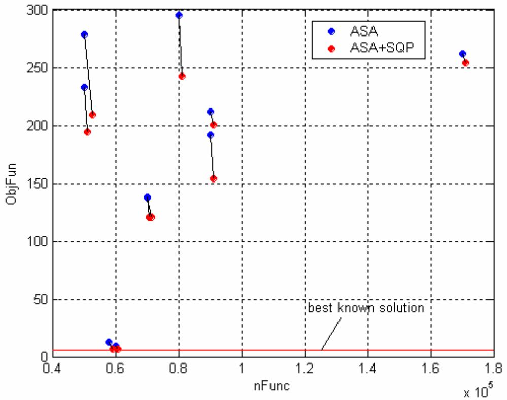
**Figure 231:** Comparison between solutions resulting from ASA runs and their improvements by means of a further local optimization process via SQP algorithm over the  $nFunc - \Delta V$  plane.
