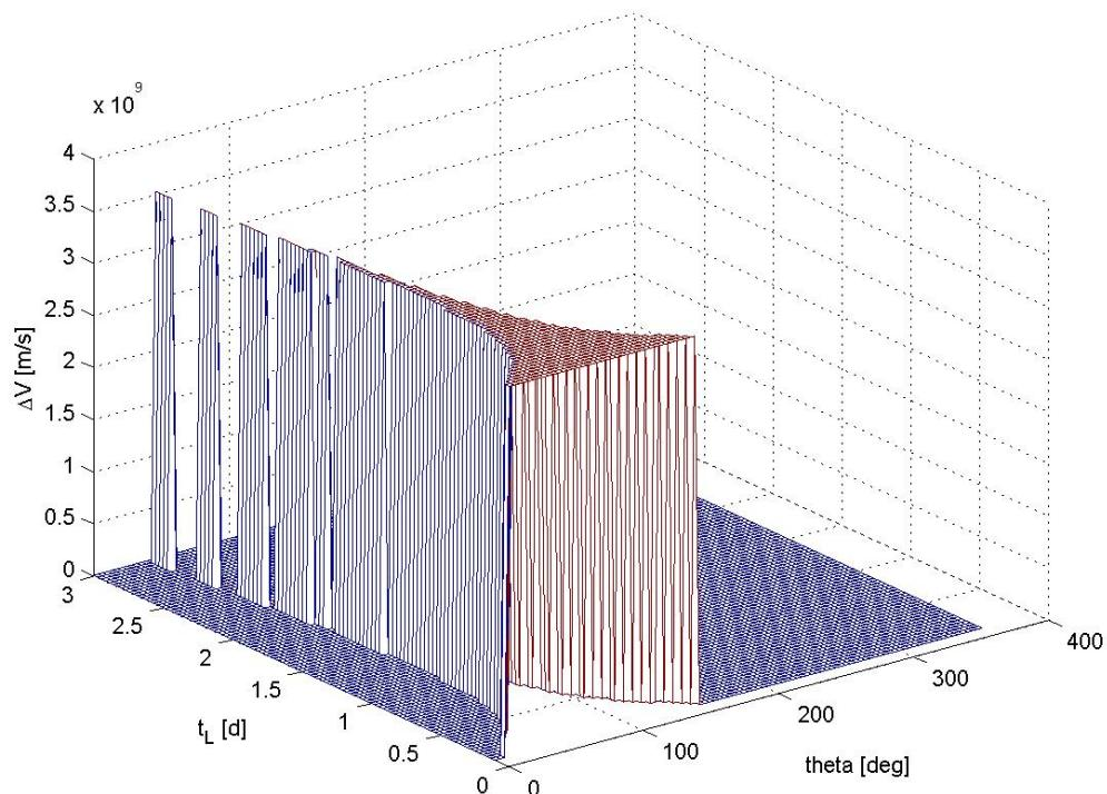
**Figure 93:** Objective function values with respect to  $\theta$  and  $t_L$ .
