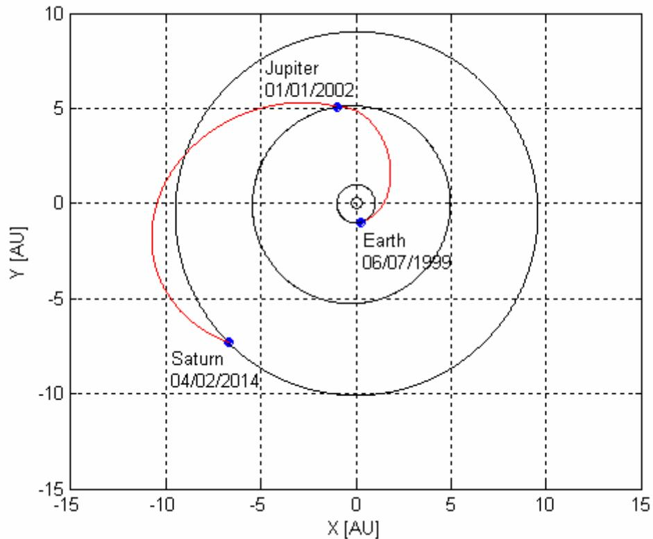
**Figure 24:** Transfer trajectory corresponding to the best solution found
