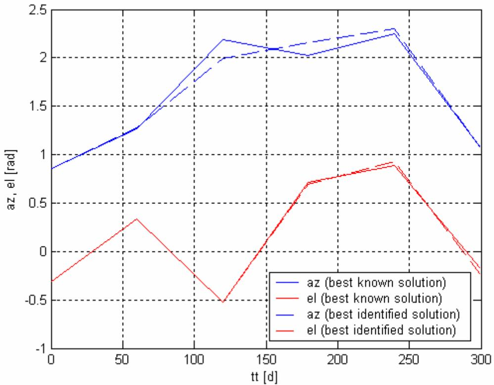
**Figure 218:** Comparison between the best identified solution and the best known solution: thrust azimuth and elevation over the transfer trajectory.
