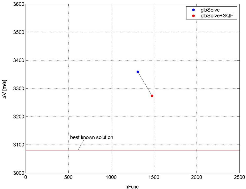
**Figure 293:** Distribution of the improved solution at the end of a local optimization process on the  $nFunc$ - $\Delta V$  plane.
