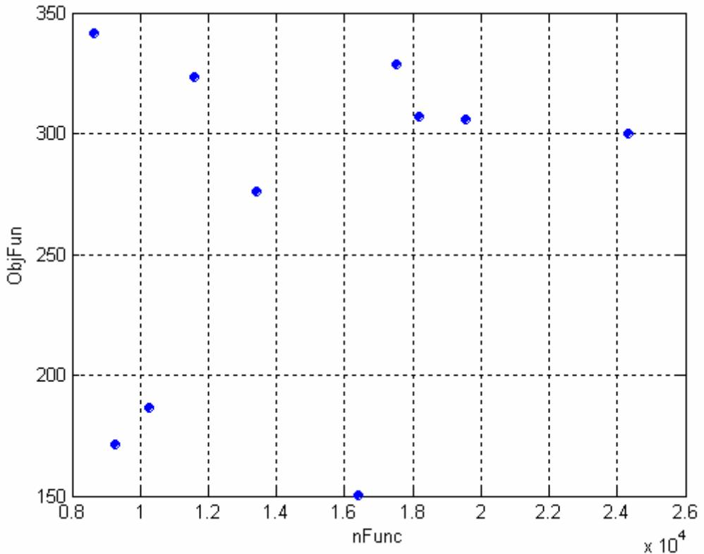
**Figure 201:** Distribution of the solutions resulting from each GAOT optimization run over the  $nFunc - \Delta V$  plane.
