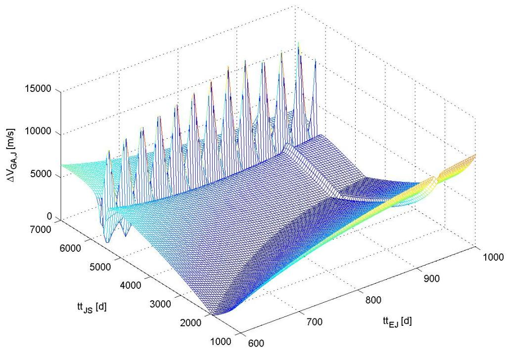
**Figure 17:**  $\Delta V_{GA,J}$  as a function of the transfer times at a fixed date of departure (-180 d).
