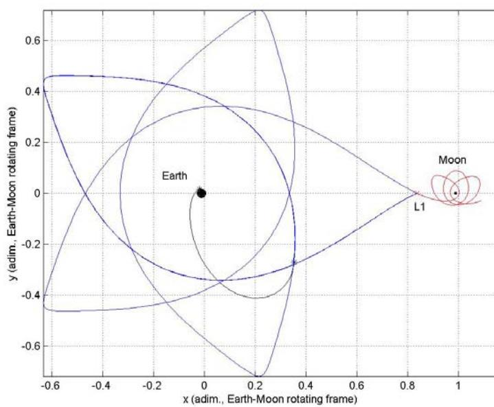
**Figure 304:** Improved solution via local optimization process: transfer trajectory.
