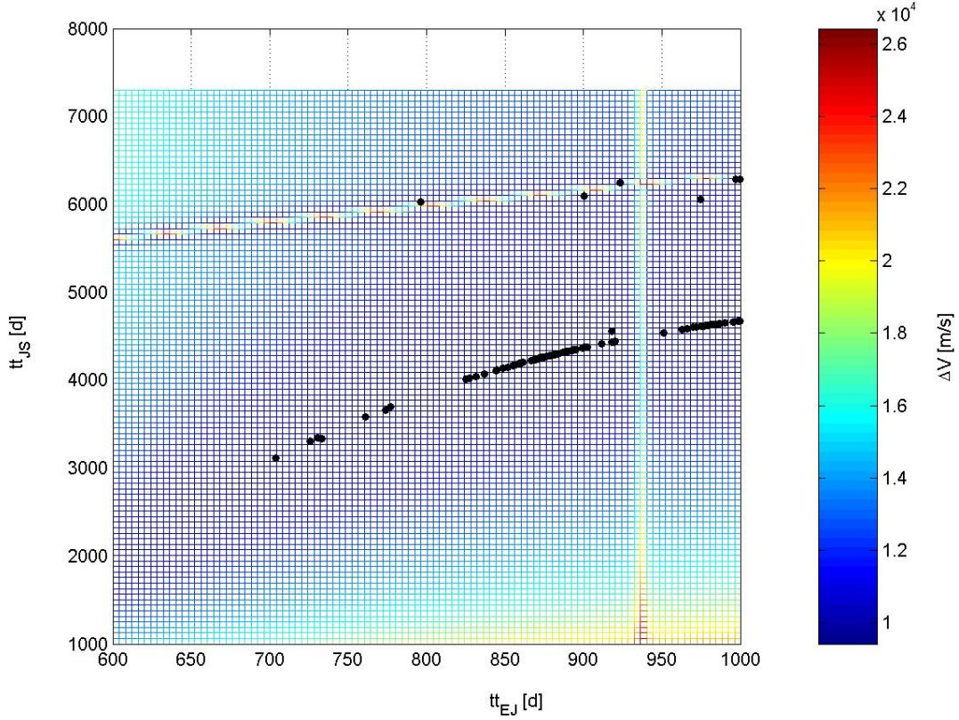
**Figure 15:** The  $\Delta V$  as a function of the transfer times at a fixed date of departure (-180 d).
