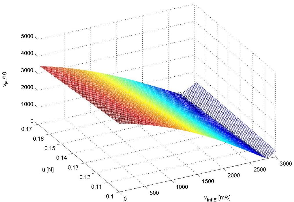
**Figure 72:**  $v_F / 10$  values with respect to the escape velocity from Earth and the thrust.
