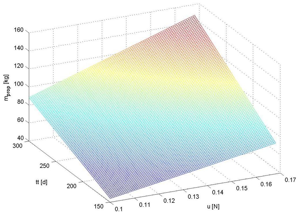
**Figure 83:** Propellant mass in the  $u - tt$  subspace.
