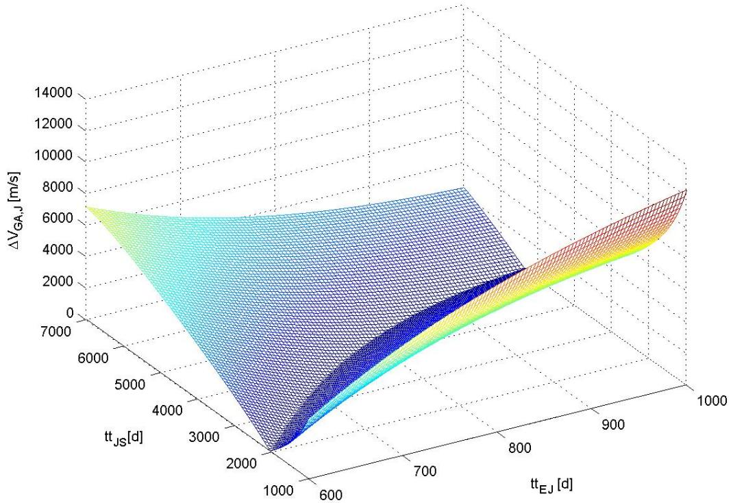
**Figure 23:**  $\Delta V_{GA,J}$  values over the transfer times search space in the two dimensional case.
