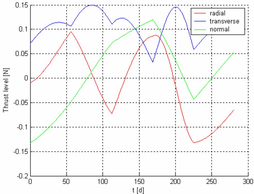
Figure 58: Thrust components in the orbital reference frame.
