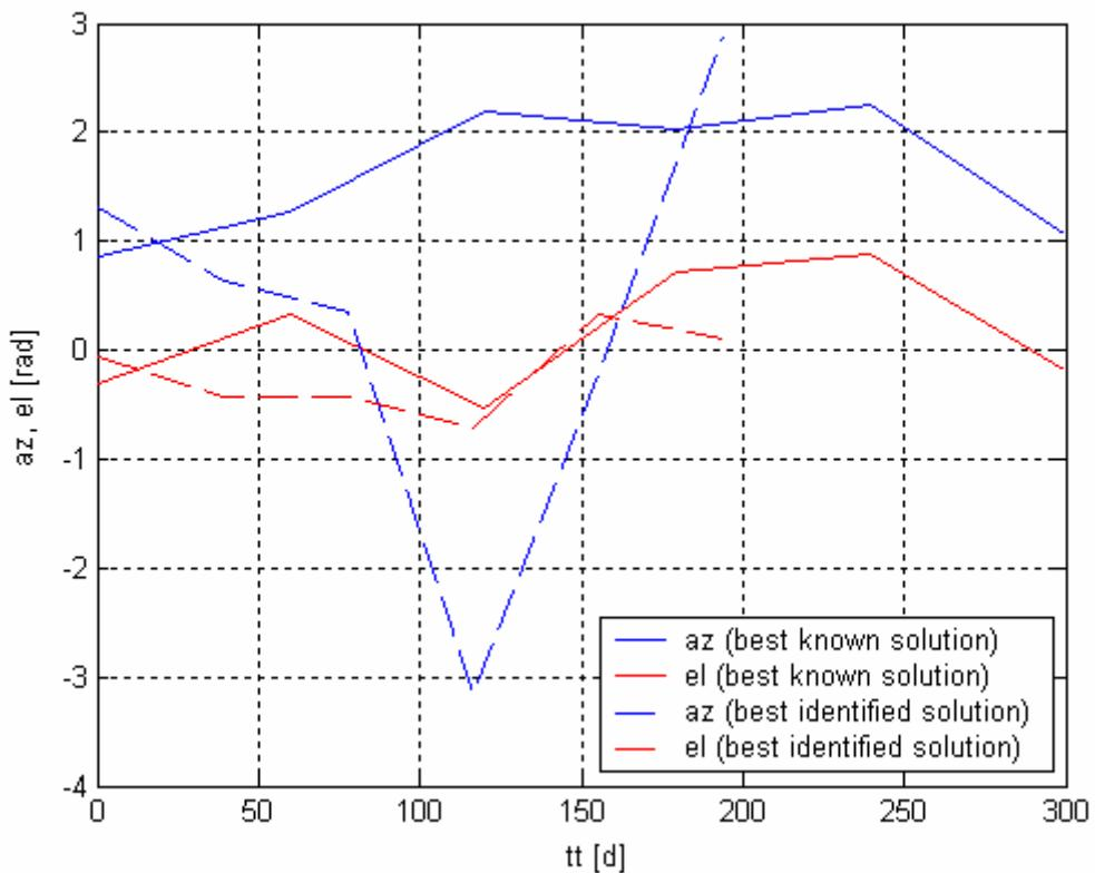
**Figure 236:** Comparison between the best identified solution and the best known solution: thrust azimuth and elevation over the transfer trajectory.
