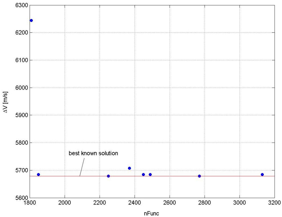
**Figure 131:** Distribution of the final solutions corresponding to each optimization run on the  $nFunc-\Delta V$  plane.
