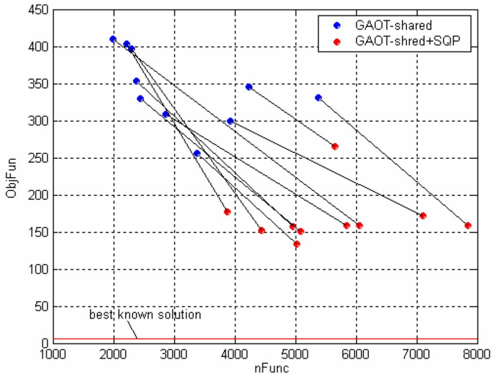
**Figure 206:** Comparison between solutions resulting from GAOT-shared runs and their improvements by means of a further local optimization process via SQP algorithm over the  $nFunc - \Delta V$  plane.
