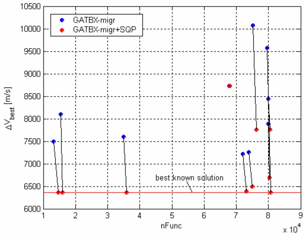
**Figure 175:** Comparison between solutions resulting from GATBX-migr runs and their improvements by means of a further local optimization process via SQP algorithm over the  $nFunc - \Delta V$  plane.
