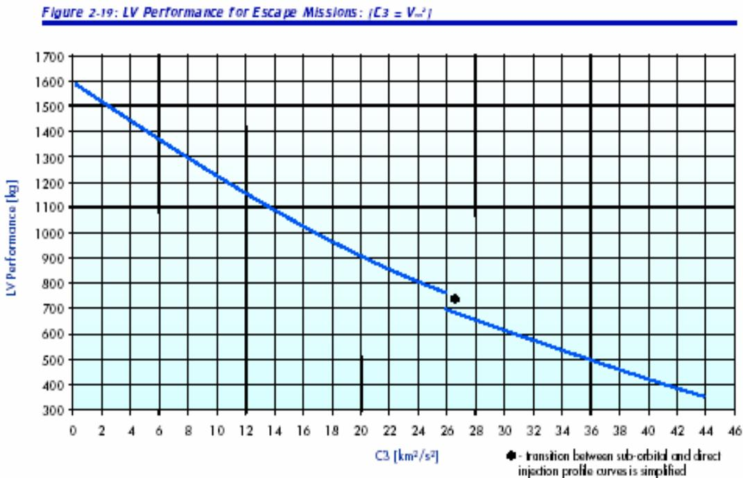
**Figure 6:** Soyuz-Fregat launcher: performance for Escape Missions.
