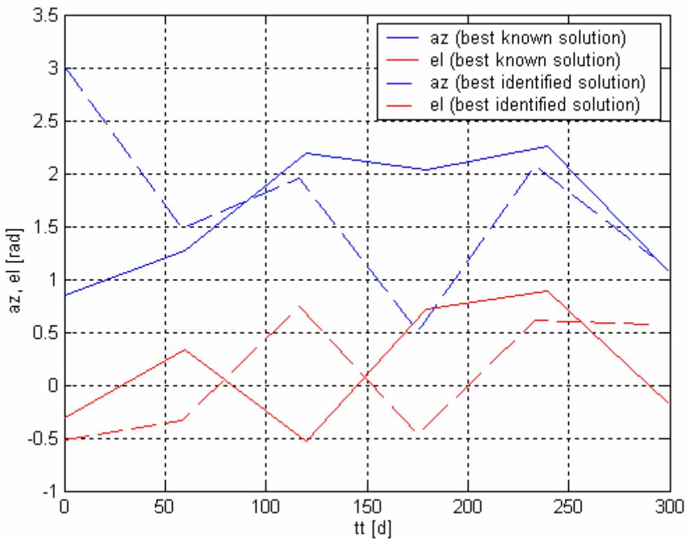
**Figure 228:** Comparison between the best identified solution and the best known solution: thrust azimuth and elevation over the transfer trajectory.
