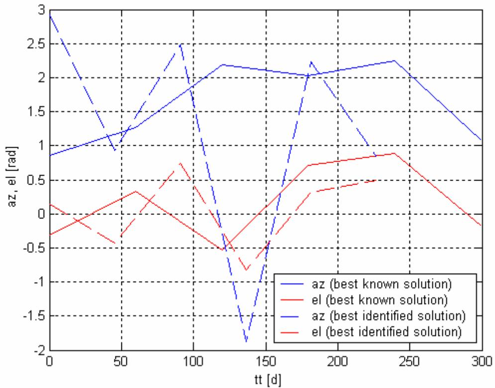
**Figure 203:** Comparison between the best identified solution and the best known solution: thrust azimuth and elevation over the transfer trajectory.
