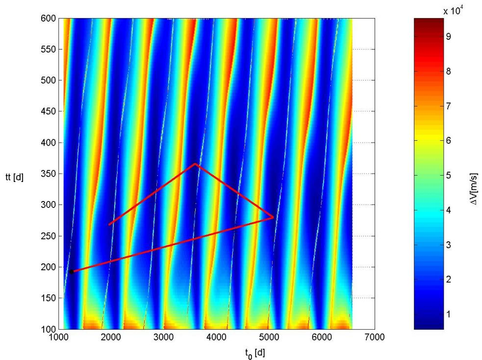
**Figure 150** - Trace of the best solution during the optimization run corresponding to an identified solution lying on the basin of attraction of the best known one.
