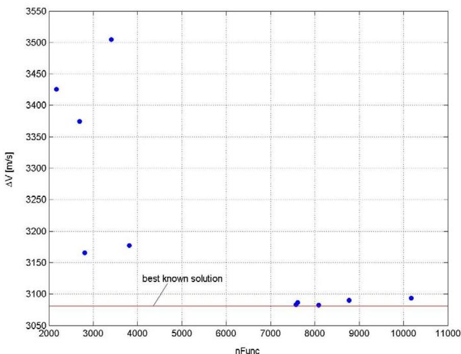
**Figure 263:** Distribution of the final solutions corresponding to each optimization run on the  $nFunc$ - $\Delta V$  plane.
