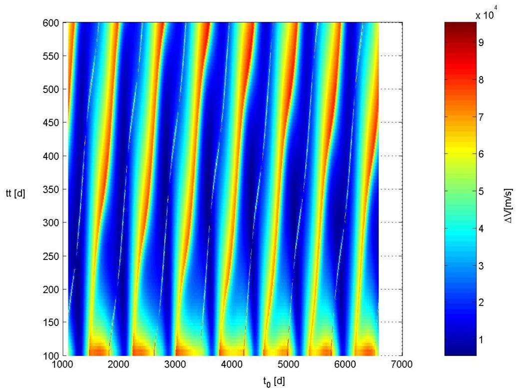
**Figure 2:** Total  $\Delta V$  for a direct impulsive Earth-Mars transfer as a function of the date of departure and the transfer time (projection on  $t_0$ - $tt$  plane)
