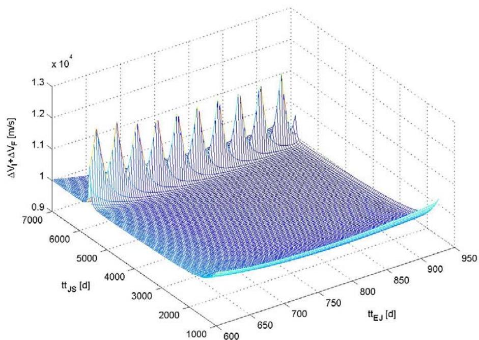
**Figure 16:**  $\Delta V_I + \Delta V_F$  as a function of the transfer times at a fixed date of departure (-180 d).
