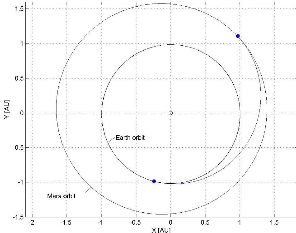
**Figure 5:** Best identified solution: transfer trajectory.
