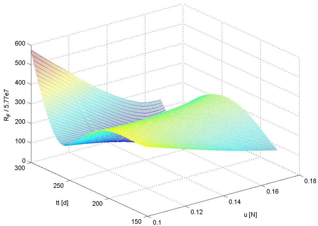
**Figure 85:**  $R_F / 5.77e7$  values with respect to the thrust level and the transfer time.
