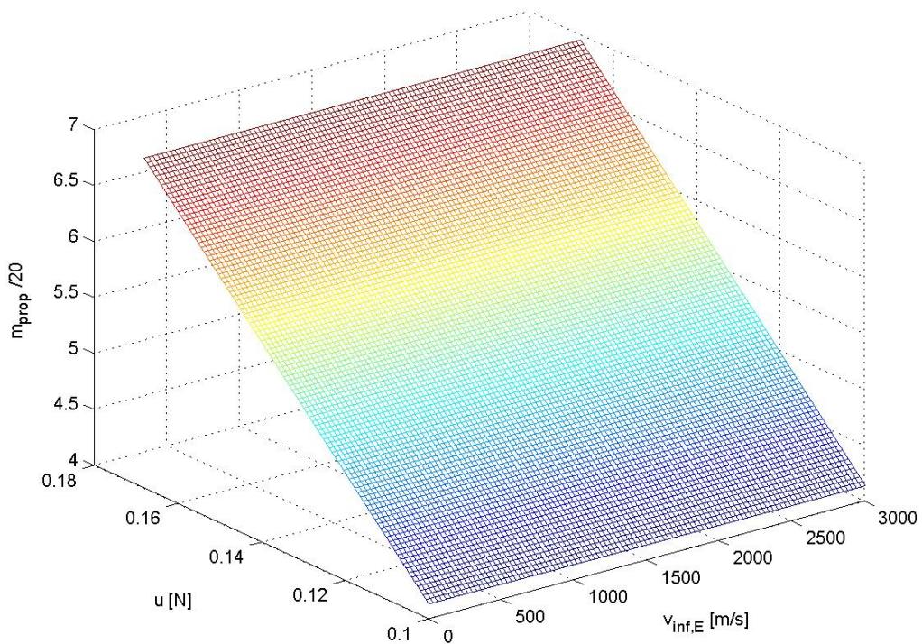
**Figure 73:**  $m_{prop}/20$  values with respect to the escape velocity from Earth and the thrust.
