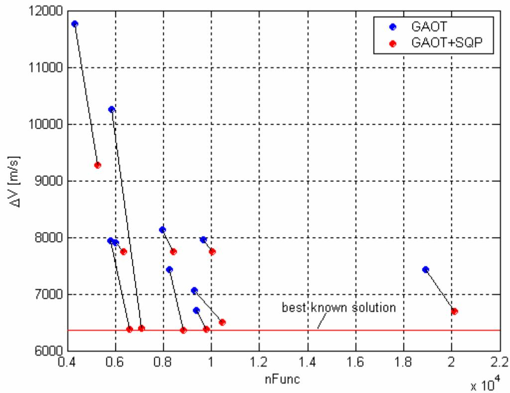
**Figure 166:** Comparison between solutions resulting from GAOT runs and their improvements by means of a further local optimization process via SQP algorithm over the  $nFunc - \Delta V$  plane.
