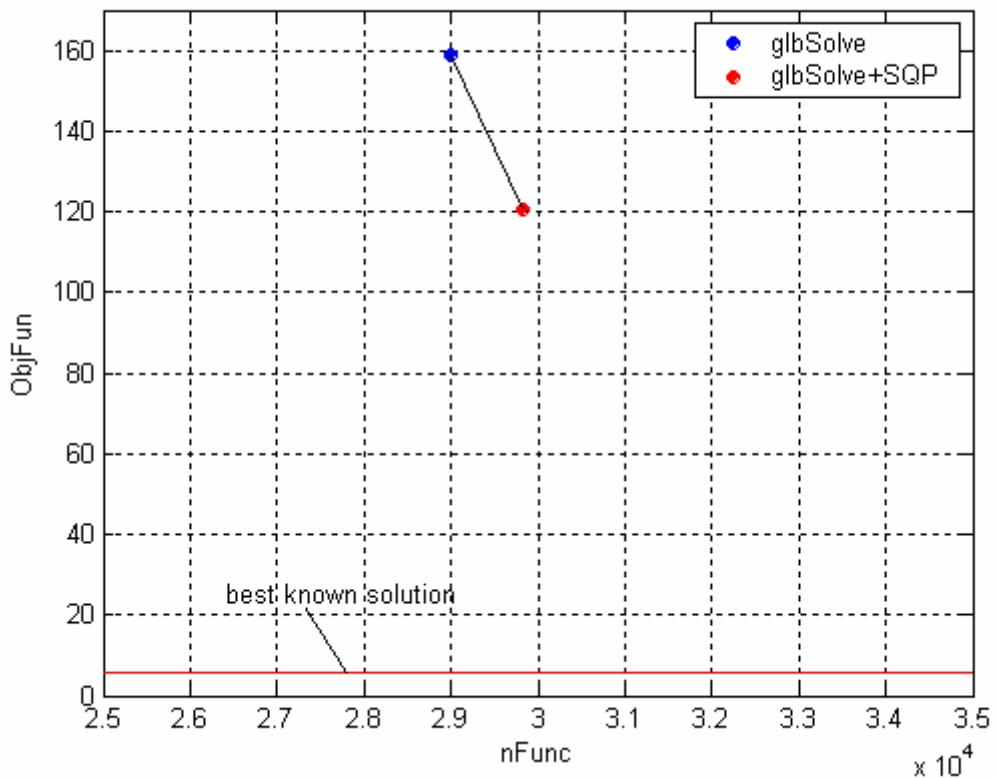
**Figure 235:** Comparison between solution resulting from glbSolve run and its improvement by means of a further local optimization process via SQP algorithm over the  $nFunc - \Delta V$  plane.
