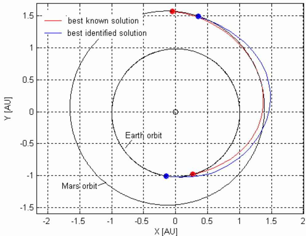
**Figure 224:** Comparison between the trajectories corresponding to the best identified solution and the best known solution.
