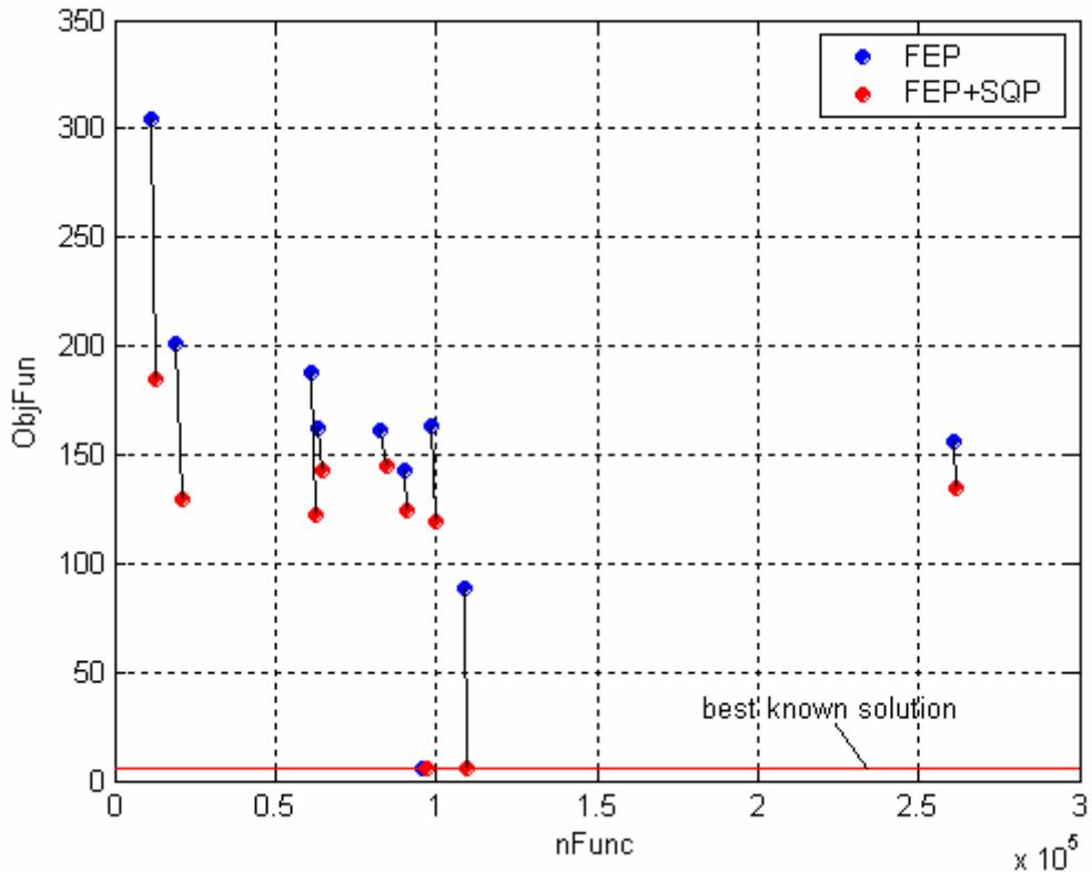
**Figure 221:** Comparison between solutions resulting from FEP runs and their improvements by means of a further local optimization process via SQP algorithm over the  $nFunc - \Delta V$  plane.
