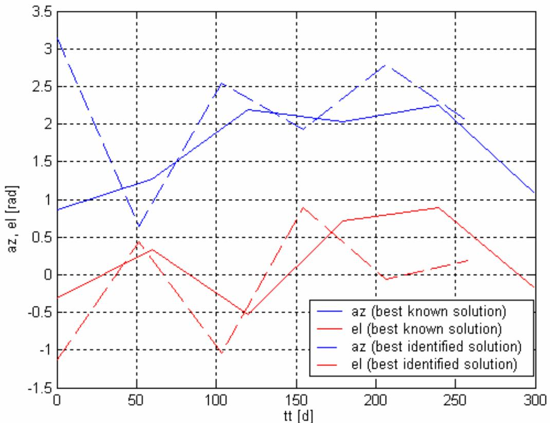
**Figure 199:** Comparison between the best identified solution and the best known solution: thrust azimuth and elevation over the transfer trajectory.
