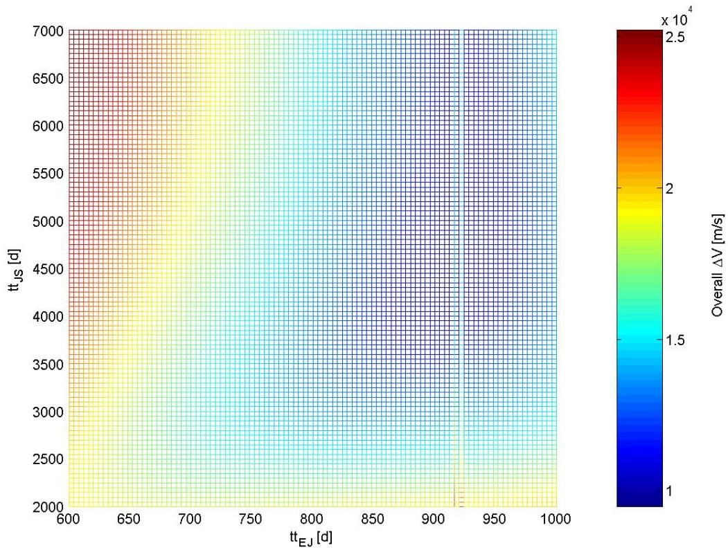
**Figure 54:** The overall  $\Delta V$  as a function of the transfer times at a fixed date of departure.
