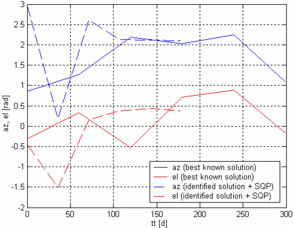
**Figure 244:** Comparison between the solution resulting from rbfSolve+SQP run and the best known solution: thrust azimuth and elevation over the transfer trajectory.
