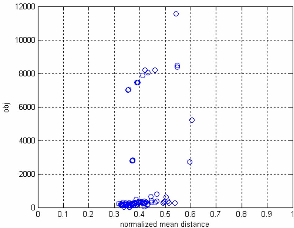
The objective function for a low thrust interplanetary mission shows again a *big-valley* structure. The mean closeness of most local optima tends to range between 0.3 and 0.5 times the hyper-diagonal magnitude. Before analysing the distribution of the local minima and verifying the existence of a *big valley* structure, let us consider the best local minimum found. The main features are listed below, together with the resulting transfer trajectory, Figure 58.
