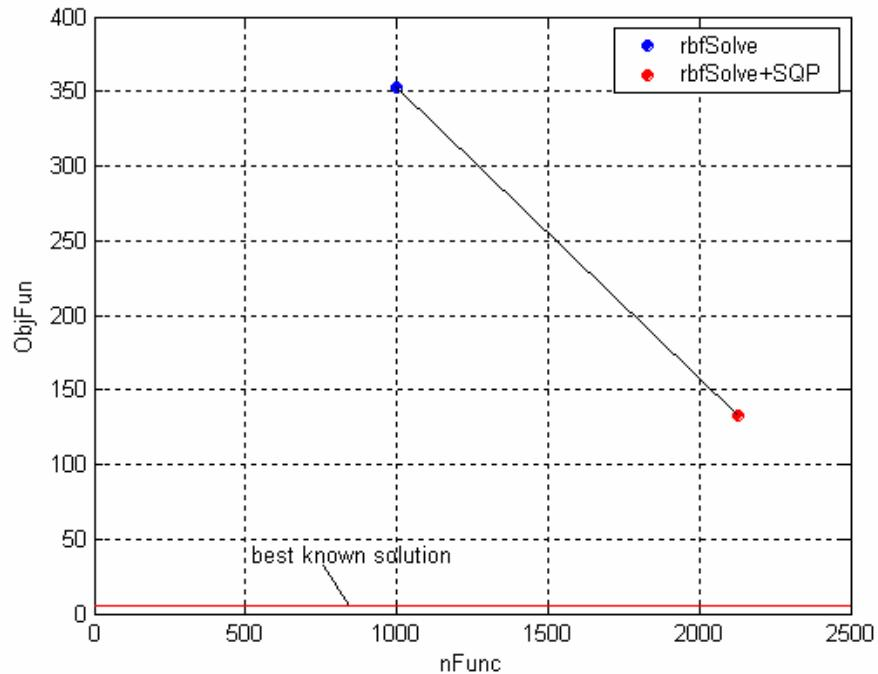
**Figure 242:** Comparison between solution resulting from *rbfSolve* run and its improvement by means of a further local optimization process via SQP algorithm over the  $nFunc - \Delta V$  plane.
