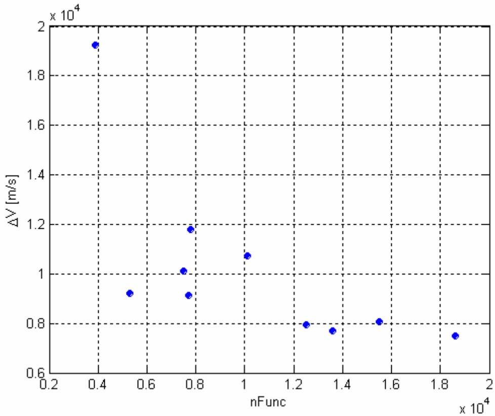
**Figure 180:** Distribution of the solutions resulting from each DE optimization run over the  $nFunc - \Delta V$  plane.
