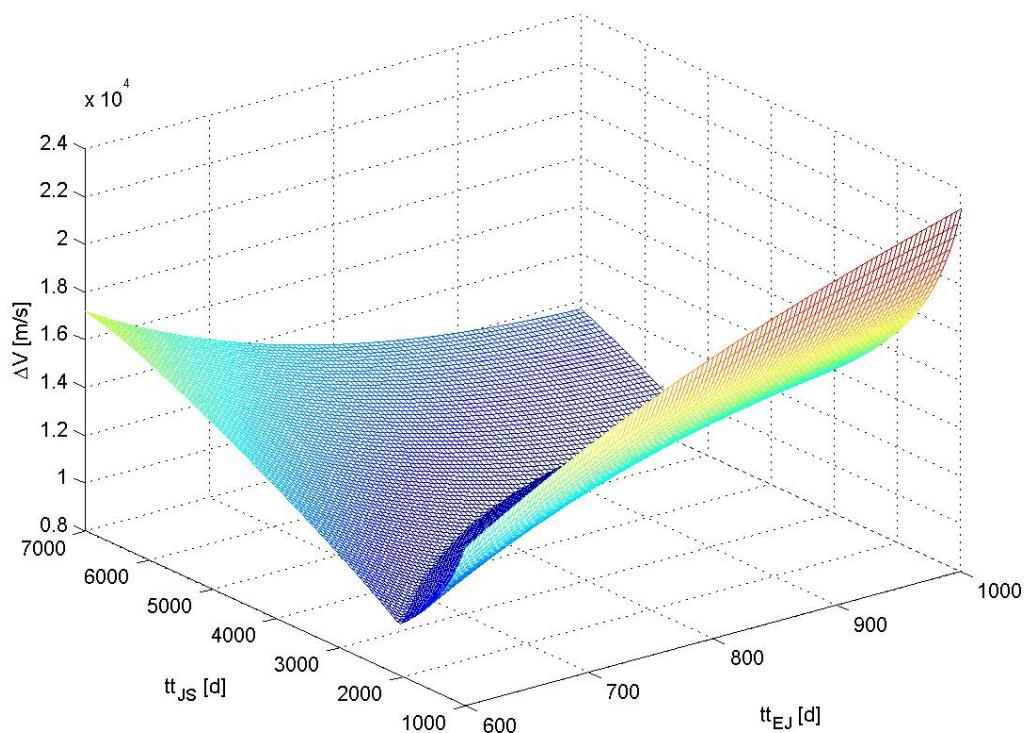
**Figure 20:** Objective function values with respect to the transfer times in a circular and coplanar planetary mathematical model.
