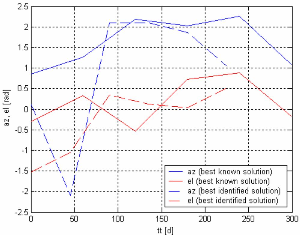
**Figure 233:** Comparison between the best identified solution and the best known solution: thrust azimuth and elevation over the transfer trajectory.
