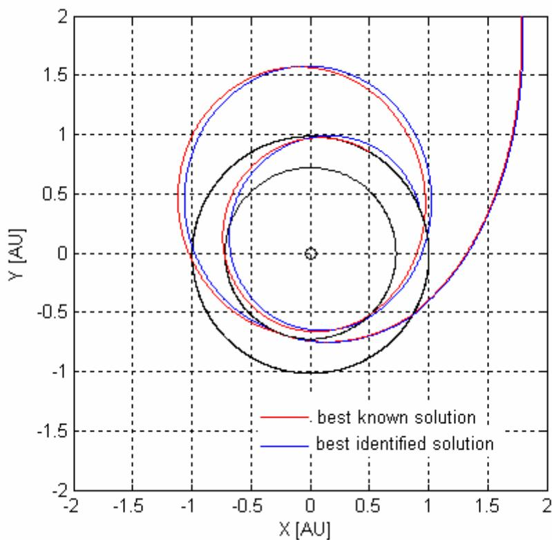
**Figure 183:** Comparison between the best identified solution and the best known solution: close up of the first phases of the interplanetary transfer reported in Figure 182.
