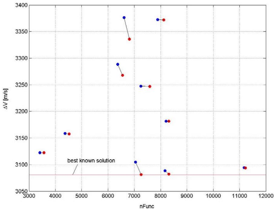
**Figure 273:** Distribution of the improved solutions at the end of a local optimization process on the  $nFunc$ - $\Delta V$  plane.
