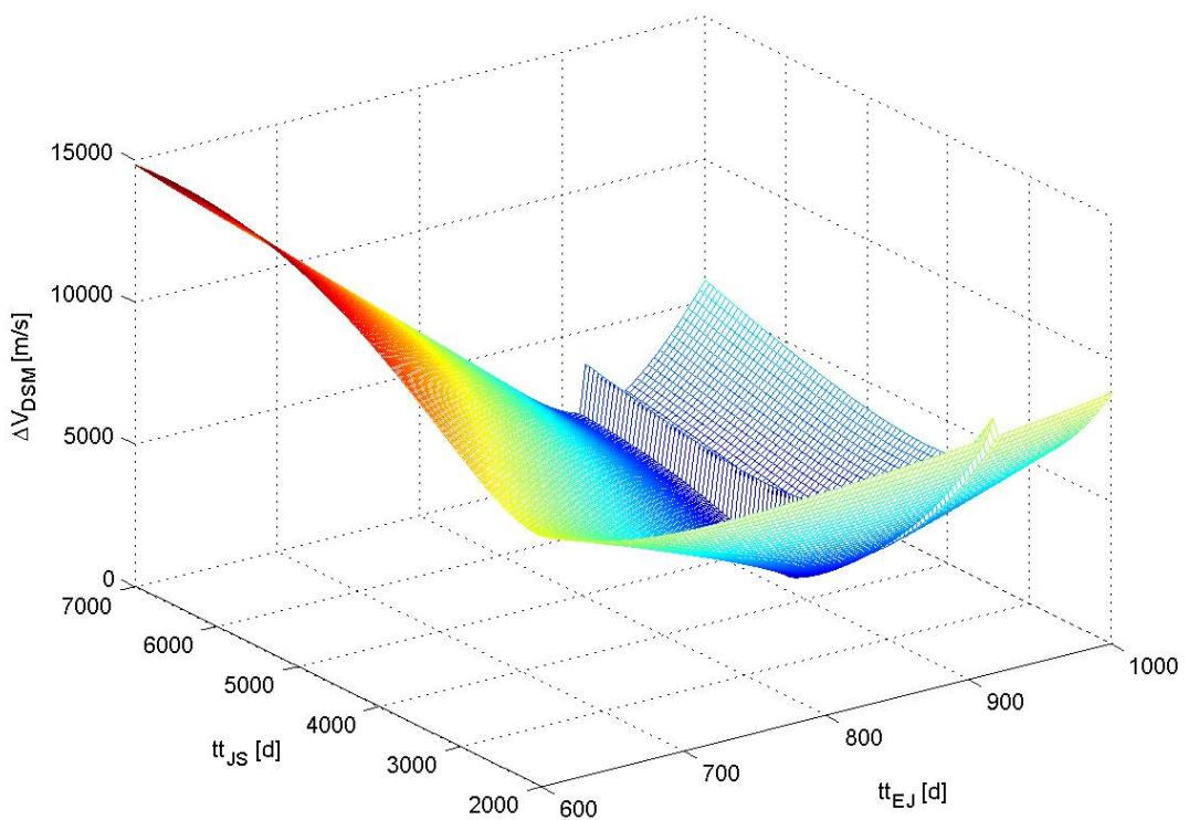
**Figure 56:**  $\Delta V_{DSM}$  as a function of the transfer times at a fixed date of departure.
