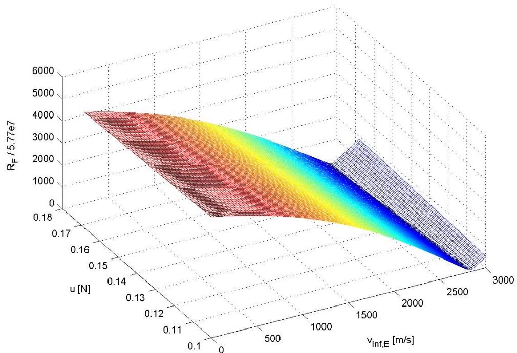
**Figure 71:**  $R_F / 5.77e7$  values with respect to the escape velocity from Earth and the thrust .
