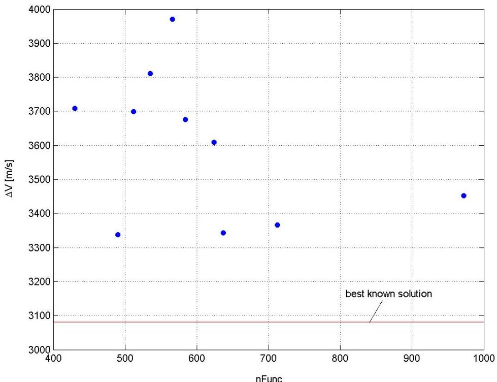
**Figure 257:** Distribution of the final solutions corresponding to each optimization run on the  $nFunc$ - $\Delta V$  plane.
