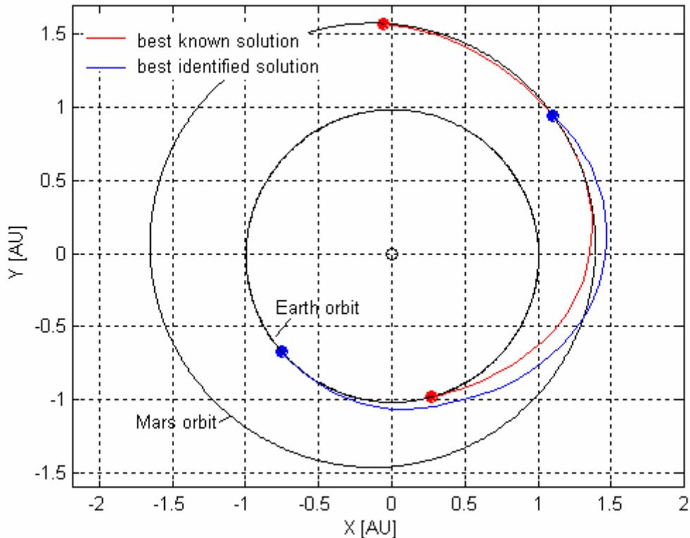
**Figure 234:** Comparison between the trajectories corresponding to the best identified solution and the best known solution.
