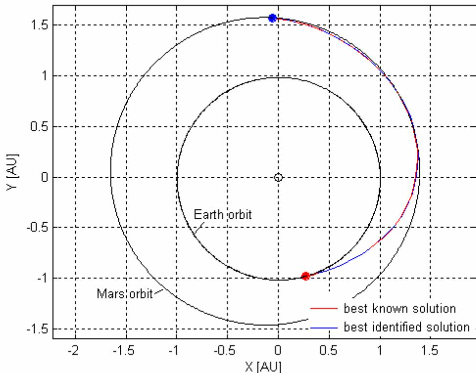
**Figure 219:** Comparison between the trajectories corresponding to the best identified solution and the best known solution.
