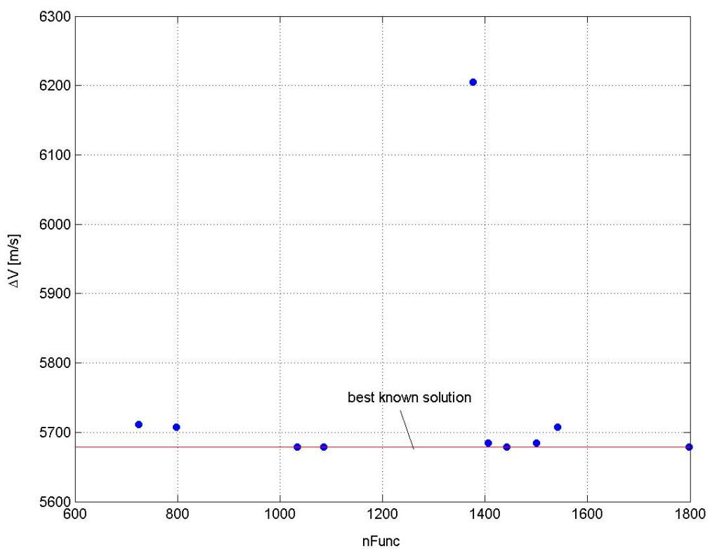
**Figure 121:** Distribution of the final solutions corresponding to each optimization run on the  $nFunc$ - $\Delta V$  plane.
