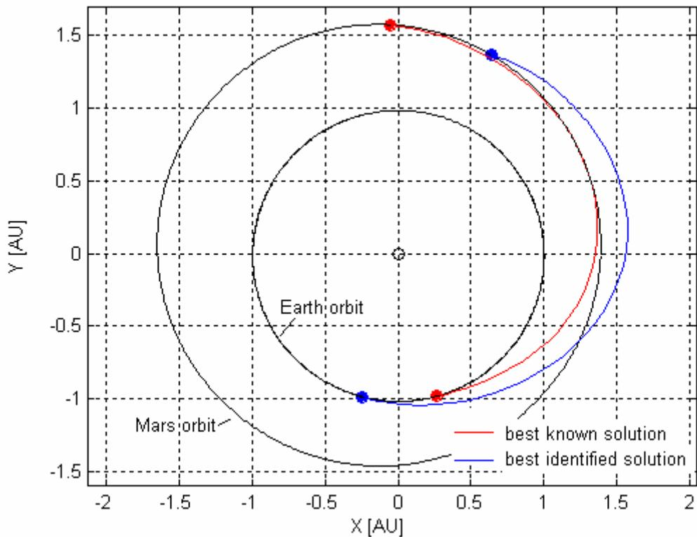
**Figure 208:** Comparison between the trajectories corresponding to the best identified solution and the best known solution.
