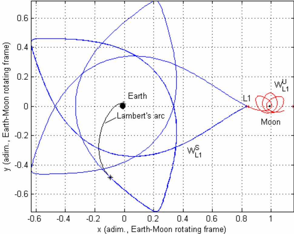
**Figure 92:** Best known solution: trajectory representation in the dimensionless Earth-Moon rotating frame.
