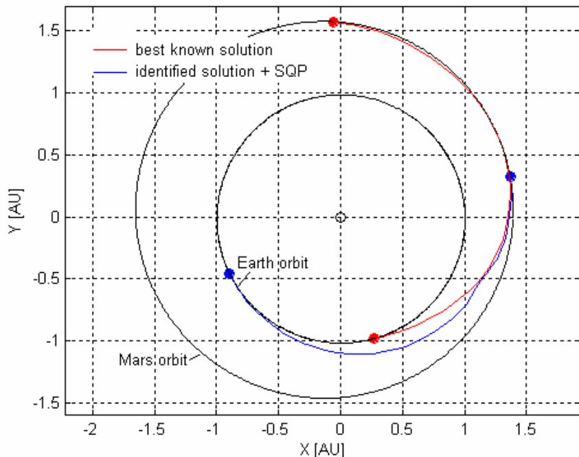
**Figure 239:** Comparison between solution resulting from MCS+SQP run and the best known solution in terms of transfer trajectory.
