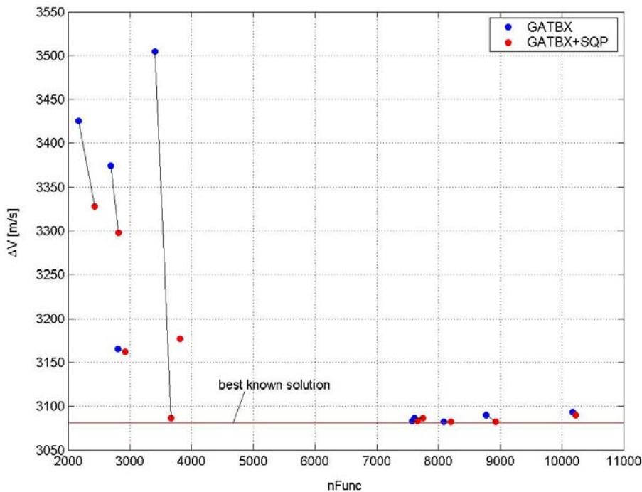
**Figure 265:** Distribution of the improved solutions at the end of a local optimization process on the  $nFunc$ - $\Delta V$  plane.
