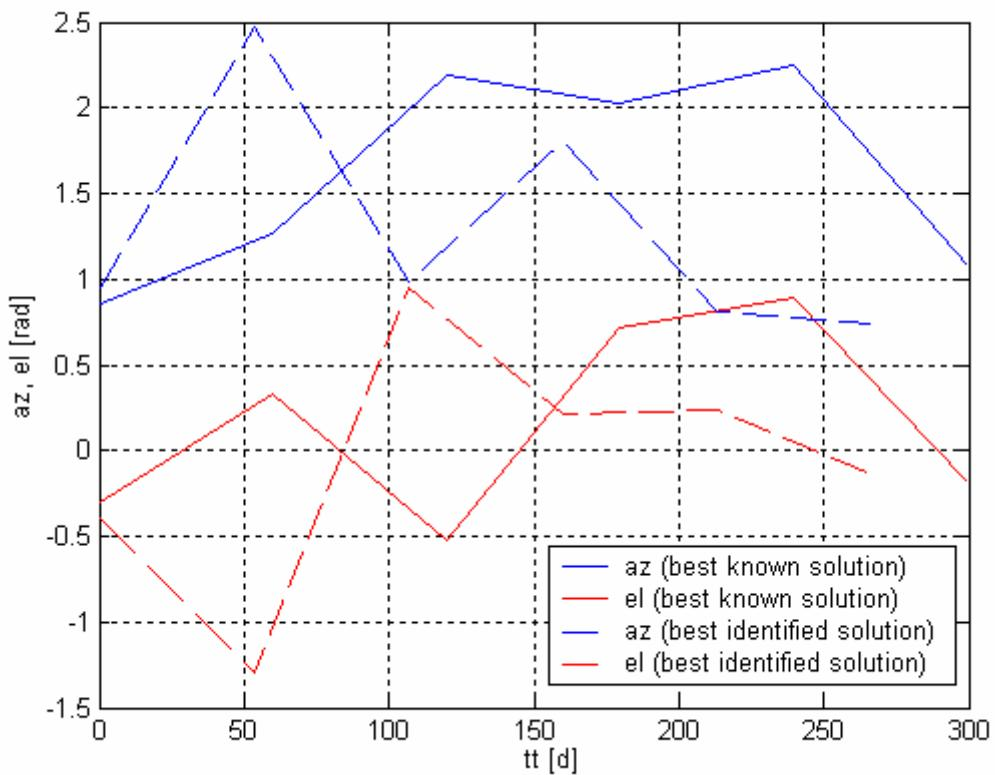
**Figure 213:** Comparison between the best identified solution and the best known solution: thrust azimuth and elevation over the transfer trajectory.
