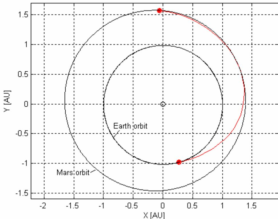
**Figure 198:** Low-thrust transfer trajectory corresponding to the best known solution.
