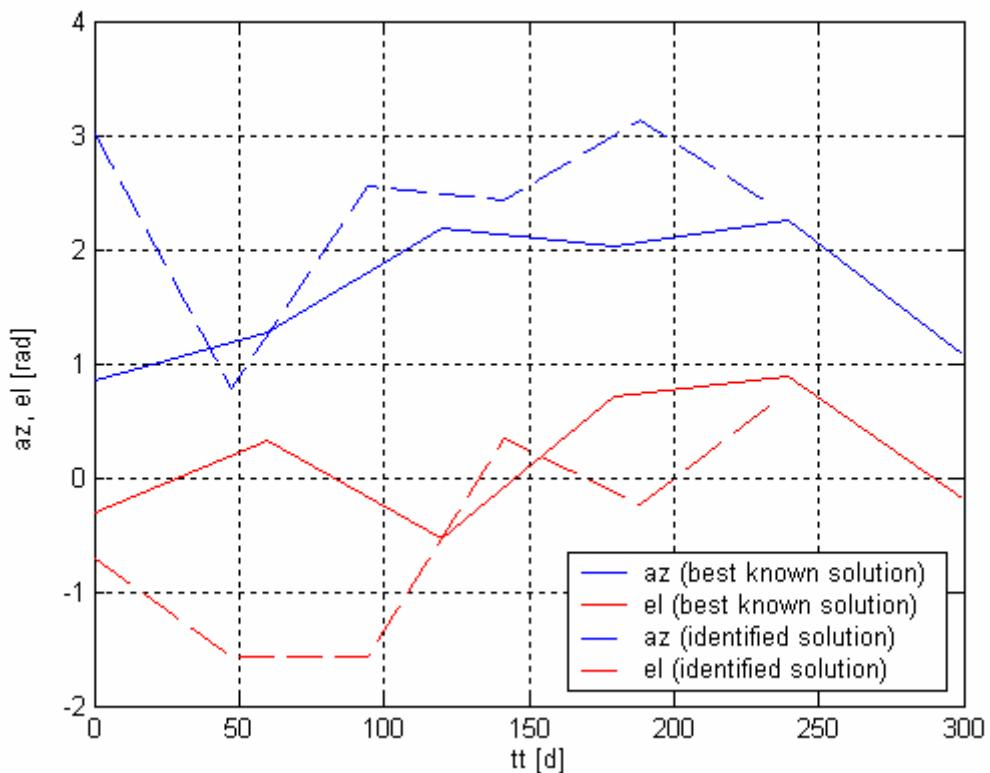
**Figure 240:** Comparison between the identified solution and the best known solution: thrust azimuth and elevation over the transfer trajectory.
