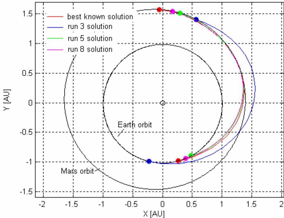
**Figure 227:** Comparison between the best known solution and solutions corresponding to run 3 and run 9.
