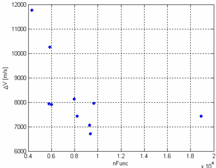
**Figure 165:** Distribution of the solutions resulting from each GAOT optimization run over the  $nFunc - \Delta V$  plane.
