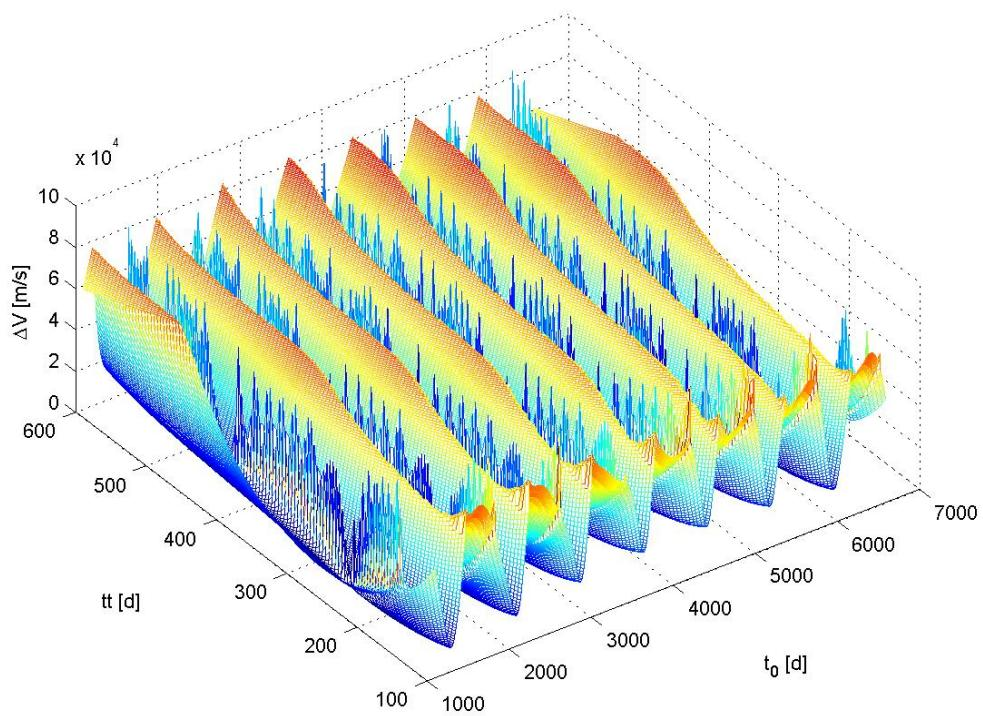
**Figure 1:** Total  $\Delta V$  for a direct impulsive Earth-Mars transfer as a function of the date of departure and the transfer time
