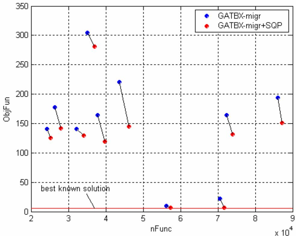
**Figure 216:** Comparison between solutions resulting from GATBX-migr runs and their improvements by means of a further local optimization process via SQP algorithm over the  $nFunc - \Delta V$  plane.
