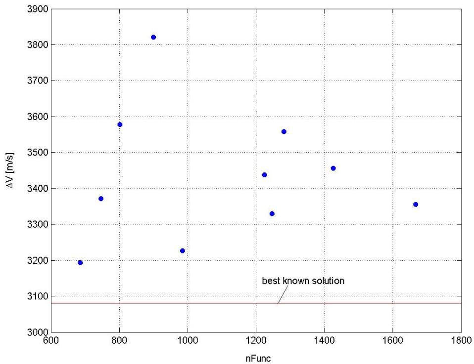
**Figure 283:** Distribution of the final solutions corresponding to each optimization run on the  $nFunc$ - $\Delta V$  plane.
