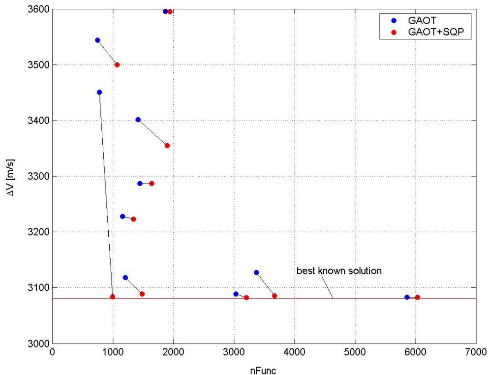
**Figure 253:** Distribution of the improved solutions at the end of a local optimization process on the  $nFunc$ - $\Delta V$  plane.
