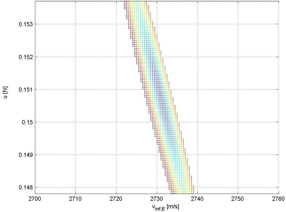
**Figure 74:** Admissible region near the best solution in the  $v_{\text{inf},E} - u$  subspace.
