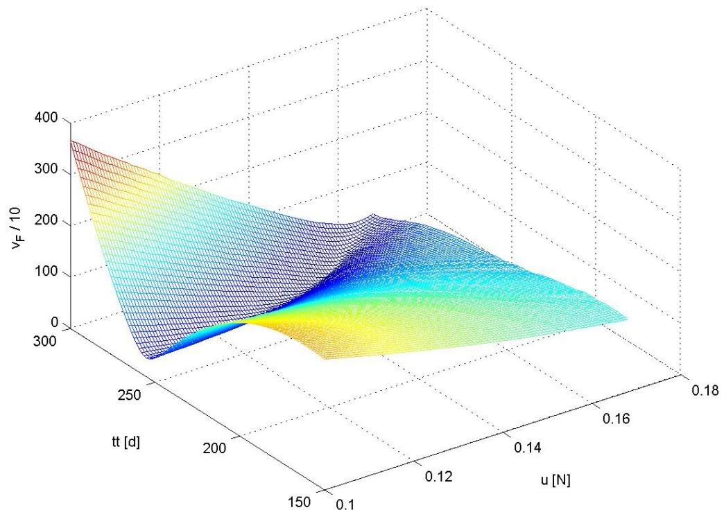
**Figure 86:**  $v_F / 10$  values with respect to the thrust level and the transfer time.
