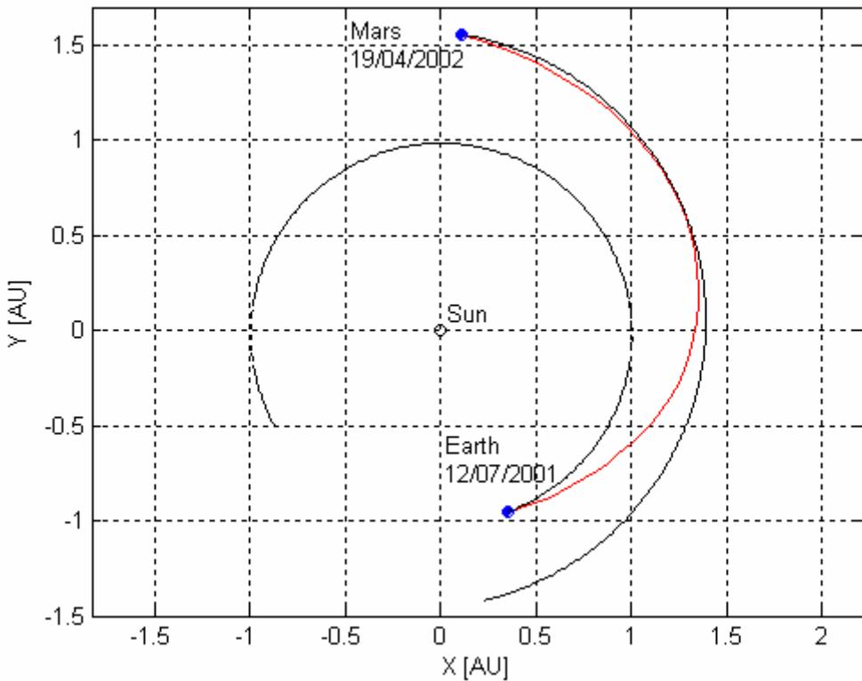
Figure 59: Transfer trajectory of the best solution in the ecliptic plane.
