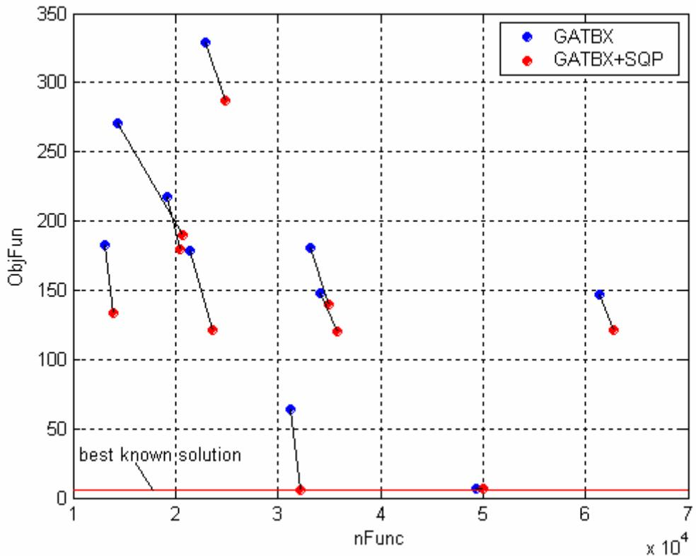
**Figure 210:** Comparison between solutions resulting from GATBX runs and their improvements by means of a further local optimization process via SQP algorithm over the  $nFunc - \Delta V$  plane.
