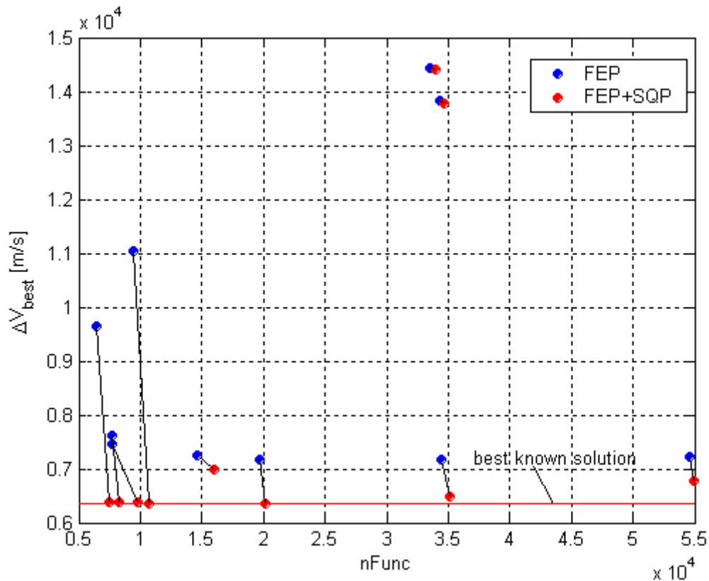
**Figure 177:** Comparison between solutions resulting from FEP runs and their improvements by means of a further local optimization process via SQP algorithm over the  $nFunc - \Delta V$  plane.
