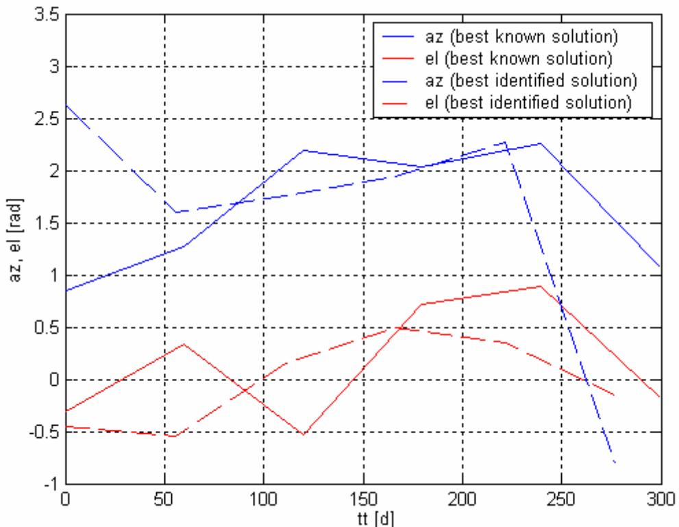
**Figure 207:** Comparison between the best identified solution and the best known solution: thrust azimuth and elevation over the transfer trajectory.
