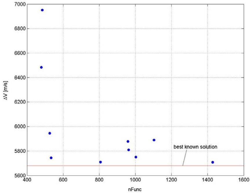
**Figure 145:** Distribution of the final solutions corresponding to each optimization run on the  $nFunc$ - $\Delta V$  plane.
