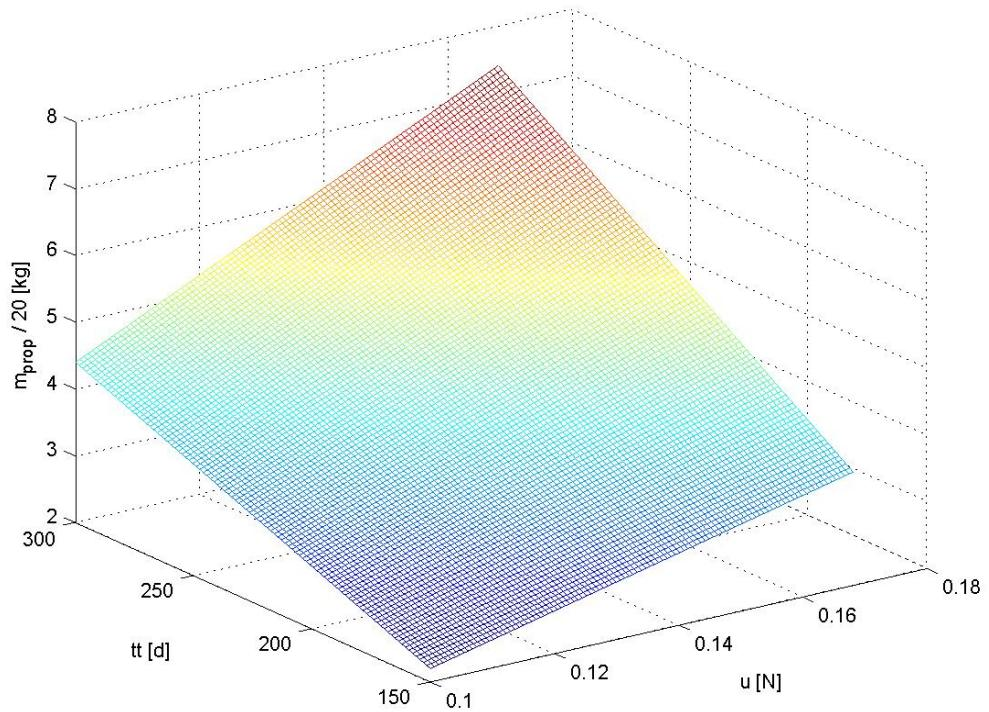
**Figure 87:**  $m_{prop} / 20$  values with respect to the thrust level and the transfer time.
