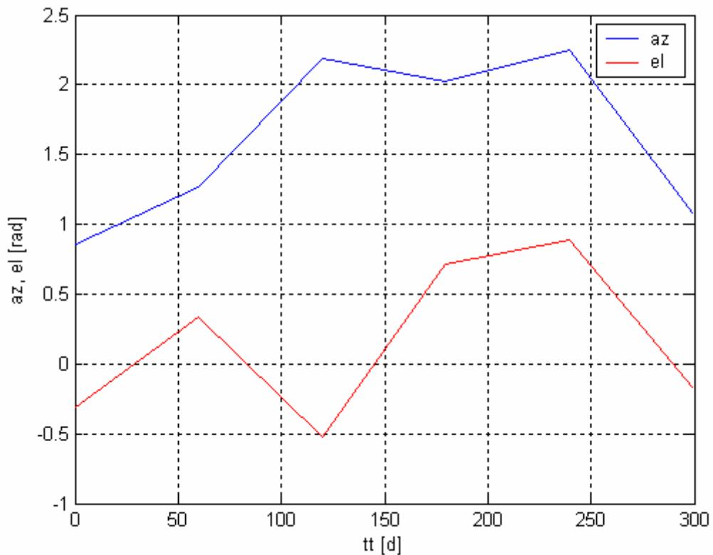
**Figure 197:** Thrust azimuth and elevation over the transfer trajectory corresponding to the best known solution.
