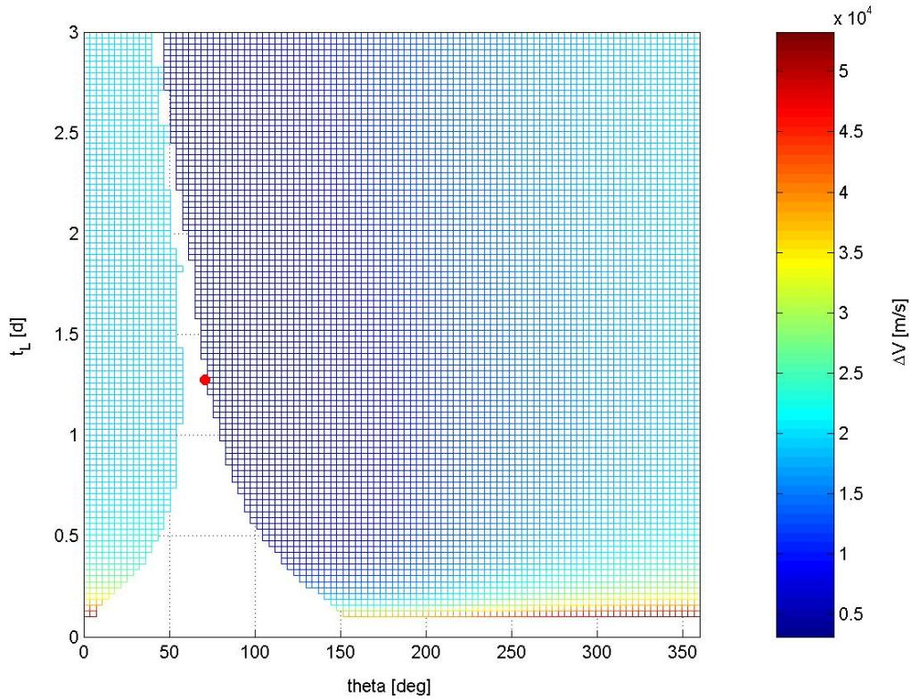
**Figure 94:** Objective function values with respect to  $\theta$  and  $t_L$ : close up of Figure 93 (the red point is the best identified solution).
