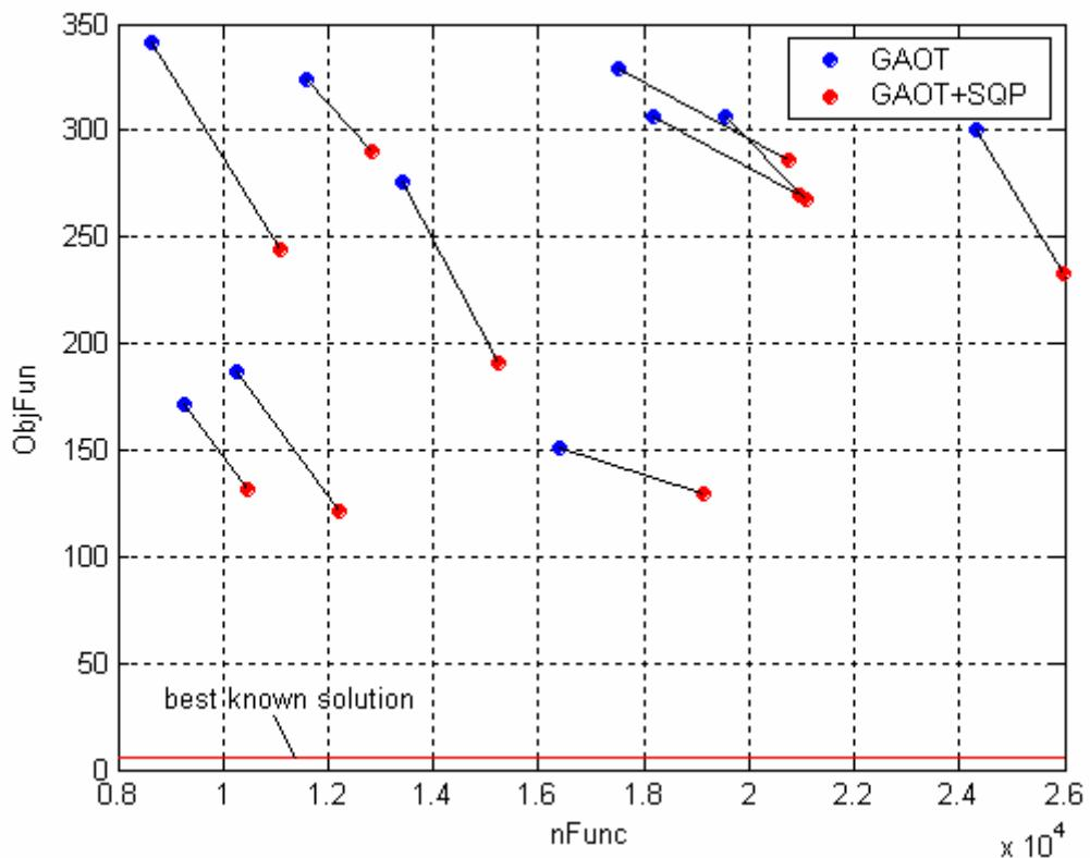
**Figure 202:** Comparison between solutions resulting from GAOT runs and their improvements by means of a further local optimization process via SQP algorithm over the  $nFunc - \Delta V$  plane.
