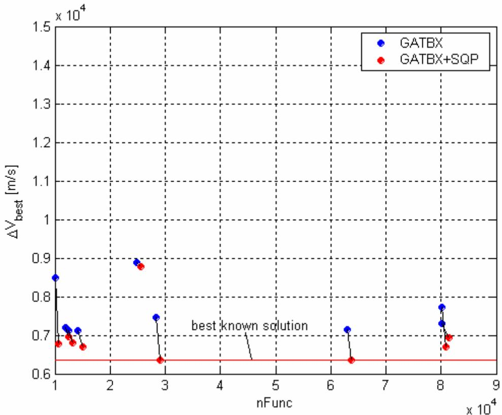
**Figure 172:** Comparison between solutions resulting from GATBX runs and their improvements by means of a further local optimization process via SQP algorithm over the  $nFunc - \Delta V$  plane.
