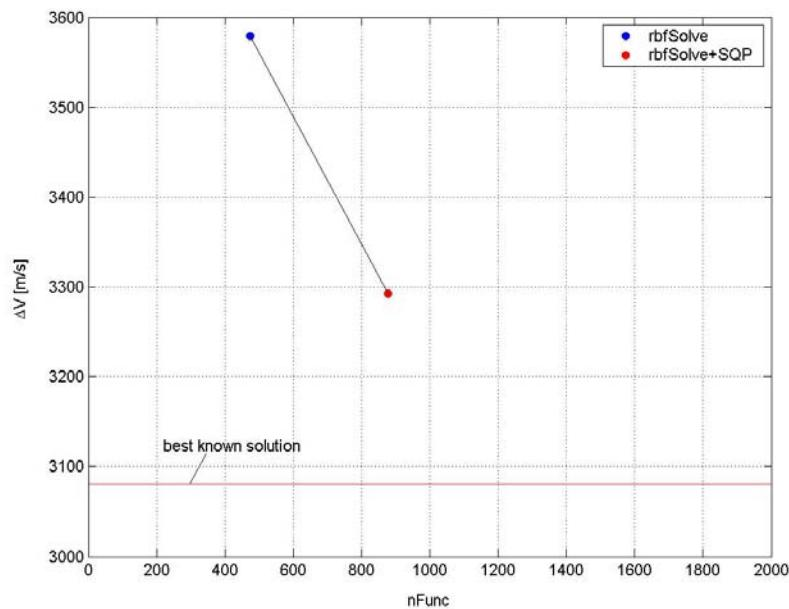
**Figure 303:** Distribution of the improved solution at the end of a local optimization process on the *nFunc*- $\Delta V$  plane.
