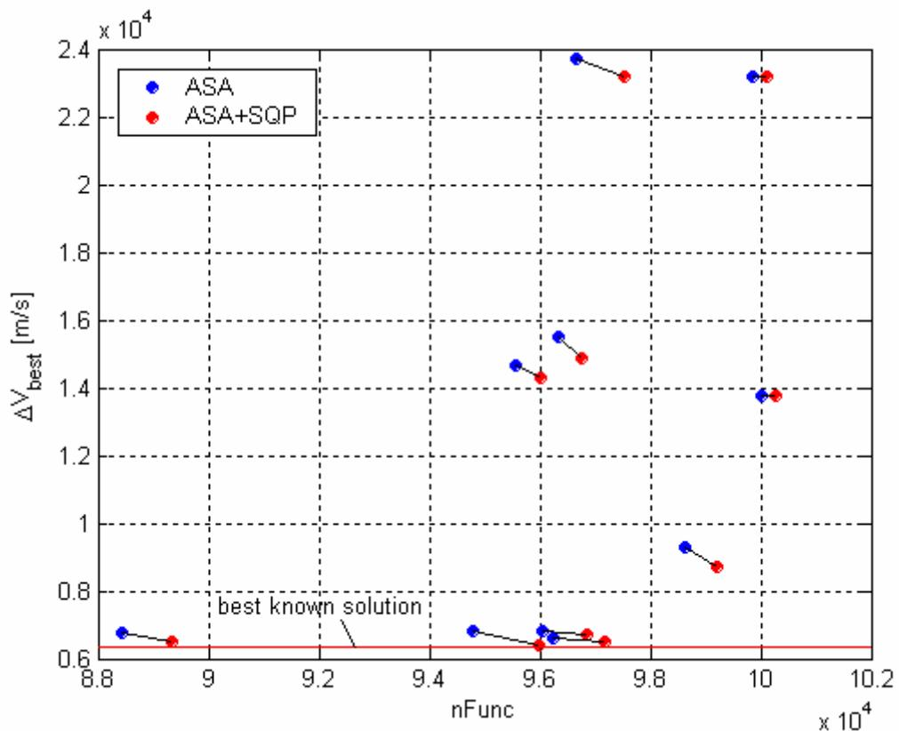
**Figure 186:** Comparison between solutions resulting from ASA runs and their improvements by means of a further local optimization process via SQP algorithm over the  $nFunc$  -  $\Delta V$  plane.
