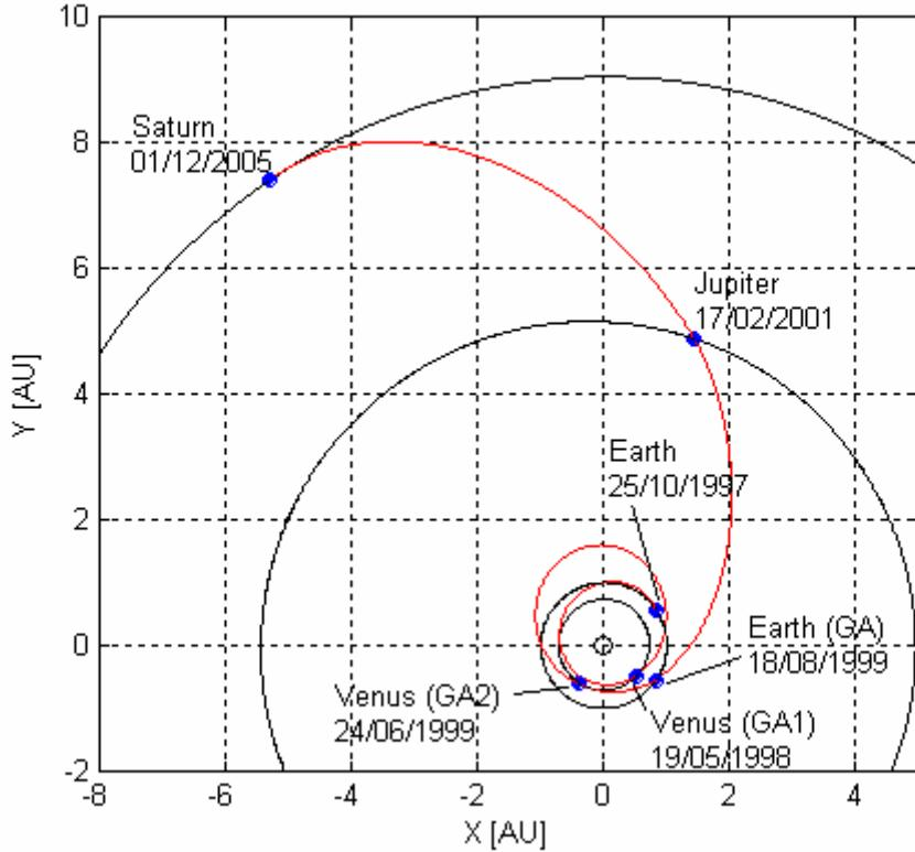
**Figure 48:** Transfer trajectory corresponding to the alternative solution.
