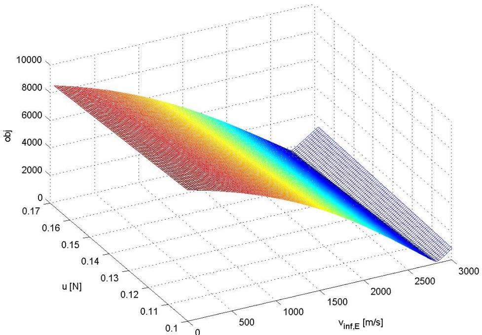
**Figure 70:** Objective function values with respect to the escape velocity from Earth and thrust.
