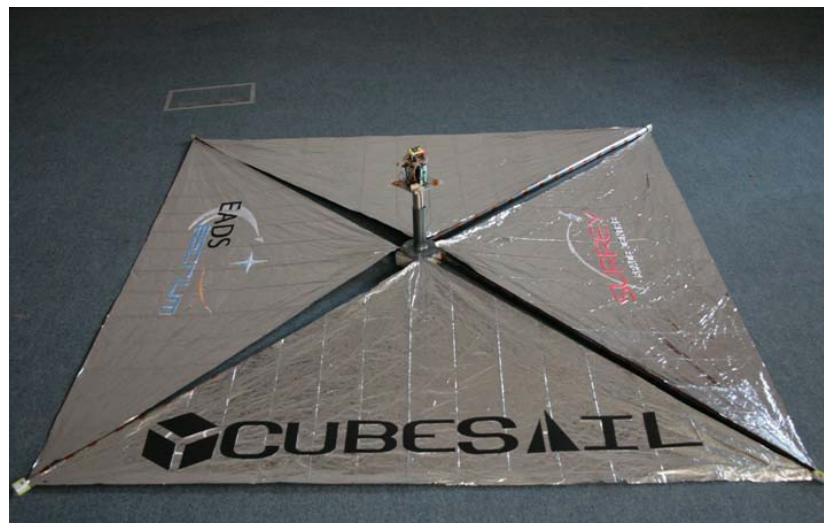
Figure 5 CubeSail 1.7m x 1.7m prototype
