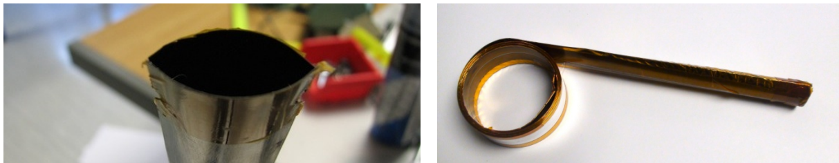
Figure 28 1.3m lenticular shaped metallic boom with Kapton tape coating
