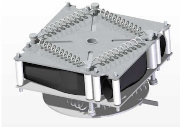
Figure 30 New Surrey boom deployment mechanism CAD drawing (left) and metallic booms manufacturing facility set-up (right)
