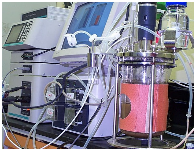
Figure 8-1. Two tank bioreactor system to produce hydrogen.
