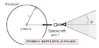
Figure 5: Spacecraft and asteroid are charged to the same polarity. Figure adapted from [7]. The engines do not need to be canted.
