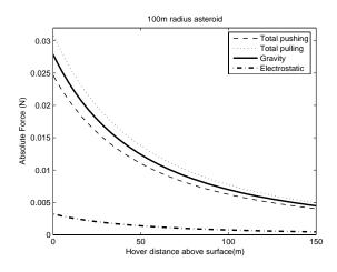
Figure 11: 100 m asteroid radius. Both asteroid and spacecraft charged to 20 kV
