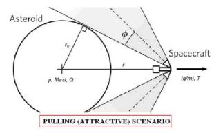
Figure 4: Spacecraft and asteroid are charged to opposite polarities. Figure adapted from [7]. The engines need to be canted.
