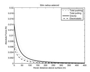
Figure 12: 50 m asteroid radius. Both asteroid and spacecraft charged to 20 kV
