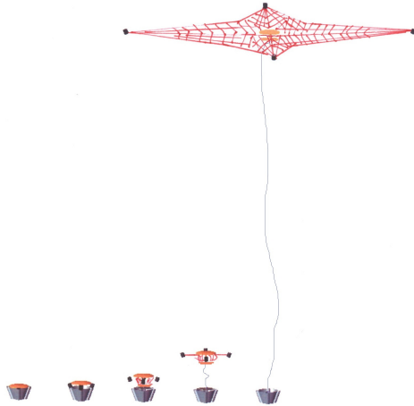
Figure 3. From left to right shows the ejection of the net from its canister.
