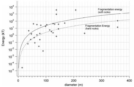
**Fig.2** Energy content of small spinning asteroids compared to the energy required to fragment them in pieces of less than 10m diameter with a buried explosive charge
