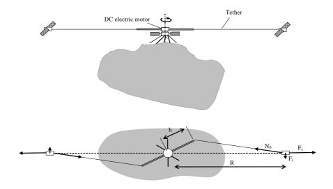
**Fig.1** Side and top view of the asteroid spin-up apparatus with represented force balance of each tethered satellite during the second phase of the spin-up process (Ft= thruster force, No= tether tension, Fc= centrifugal force)
