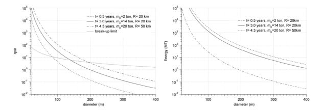
**Fig.3** Achievable asteroid spin rate and kinetic energy at mission end. Each end spacecraft is equipped with an ion propulsion thruster with 10 kW of power, 0.5N of thrust and 1900s of specific impulse.
