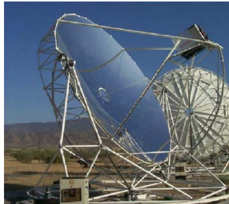
Figure 4.1/2: Example of 10 kWe thermal generator (Schlaich Bergermann & Partner source)
