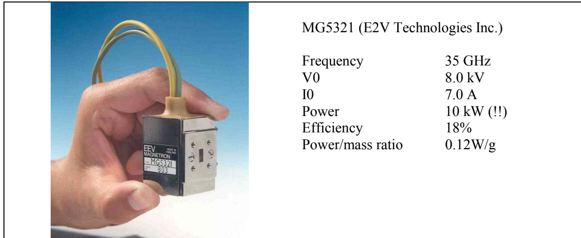
Figure 7/9: Miniature magnetron developed by E2V Technologies, and available data
