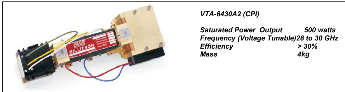
Figure 7/17: VTA-6430A2 from CPI and corresponding data. Notice the high power/mass ratio of this device.
