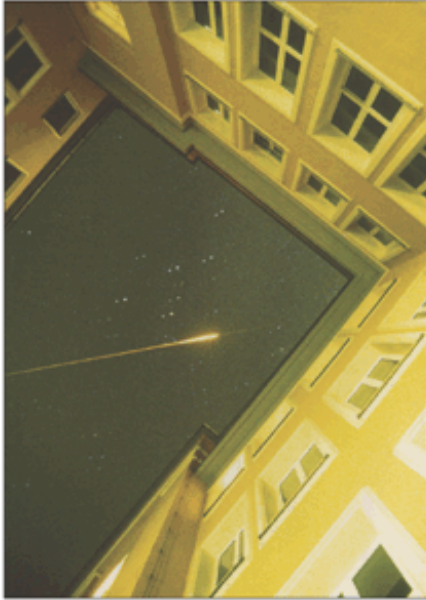
Fig. 2: Photograph of a terawatt femtosecond laser pulse directed into the sky from the University of Jena. The pulses form filaments of white light that can extend more than 20 km into the atmosphere [6]
