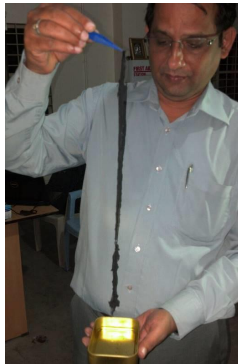
Figure 2: As-produced high purity Single Walled Carbon Nanotubes from NoPo Private Limited
